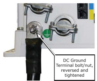
Figure 2-17, Large Ground Wire Connected to MS-E Series
