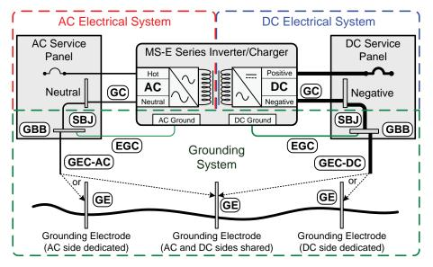
Figure 2-10, Grounding System for MS-E Series
