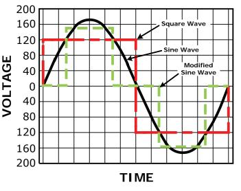
Figure C-1, AC Waveforms
