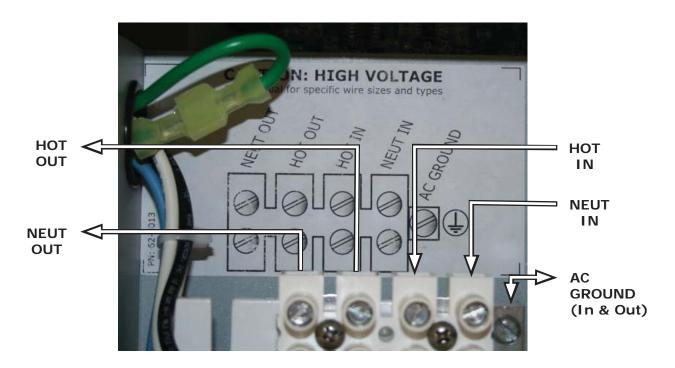
Figure 2-8, AC Terminal Block
