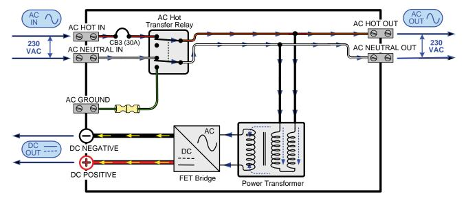
Figure 3-2, Power Flow – Standby Mode
