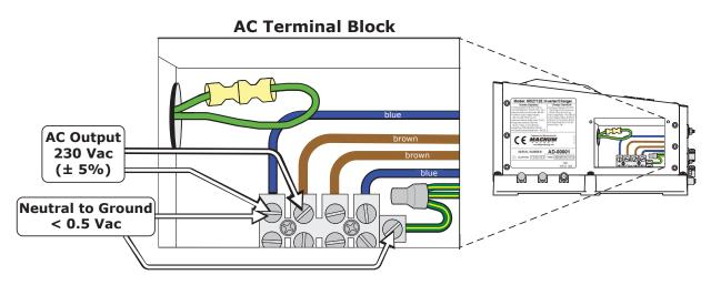
Figure 2-19, AC Voltage Checks
