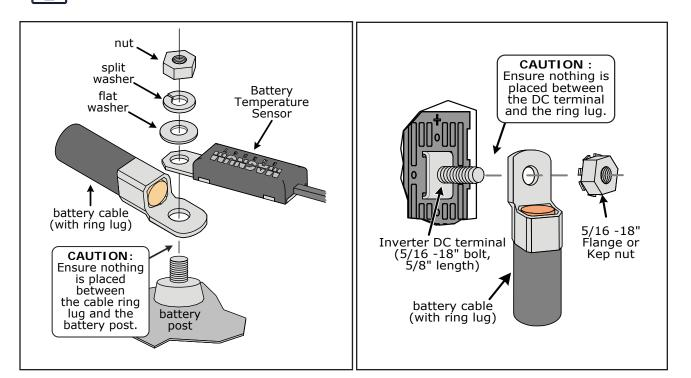
Figure 2-5, Battery Hardware Installation
