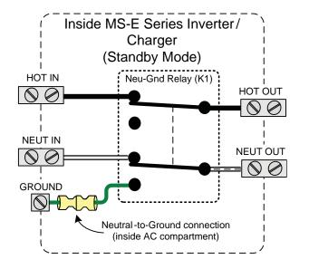
Figure 2-15, Neutral-to-Ground Connection (Standby Mode)
