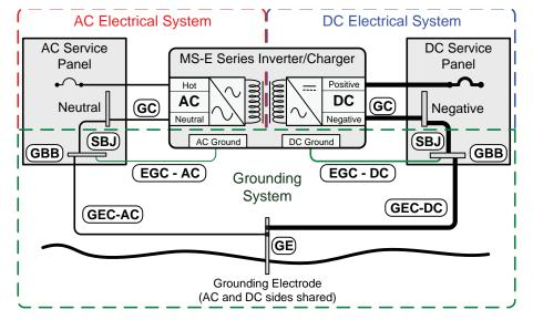
Figure 2-12, Multiple Connections to DC Ground Rod (Method 2)
