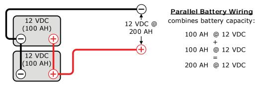
Figure B-2, Parallel Battery Wiring
