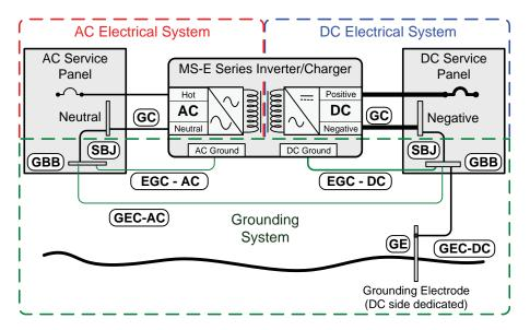
Figure 2-13, Single Connection to DC Ground Rod (Method 3)
