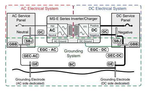
Figure 2-11, Multiple Connections to DC Ground Rod (Method 1)
