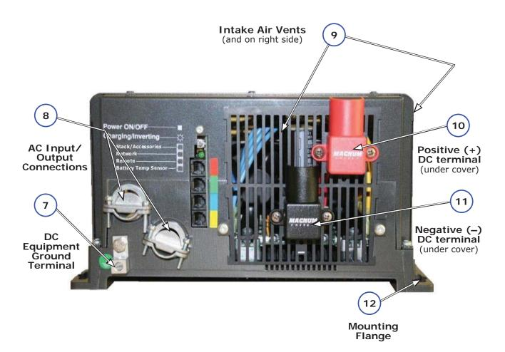
Figure 1-2, Electrical Connection Points
