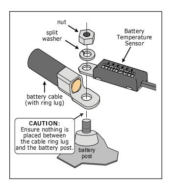
Figure 2-5, Battery Hardware Installation
