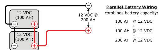
Figure B-2, Parallel Battery Wiring
