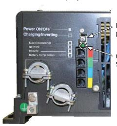
Power ON/OFF pushbutton switch
