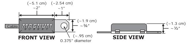
Figure 2-7, Battery Temperature Sensor
