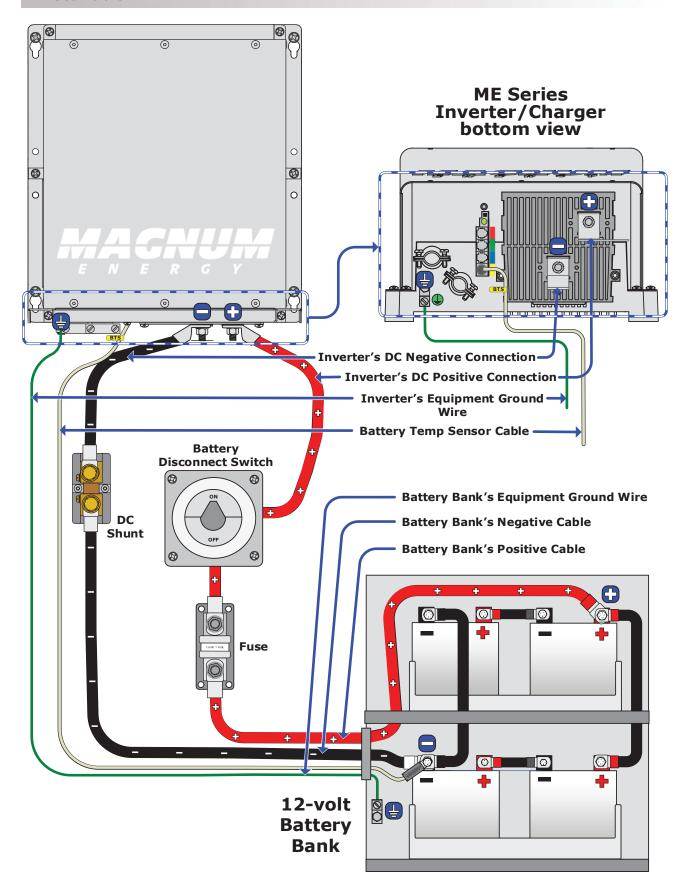
Figure 2-4, DC and Battery Temperature Sensor Wiring
