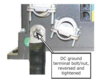
Figure 2-16, Connecting a Large DC Ground Wire
