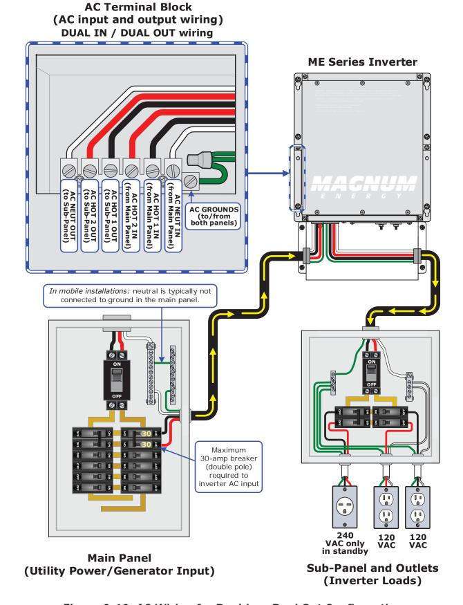
Figure 2-13, AC Wiring for Dual In – Dual Out Configurations
