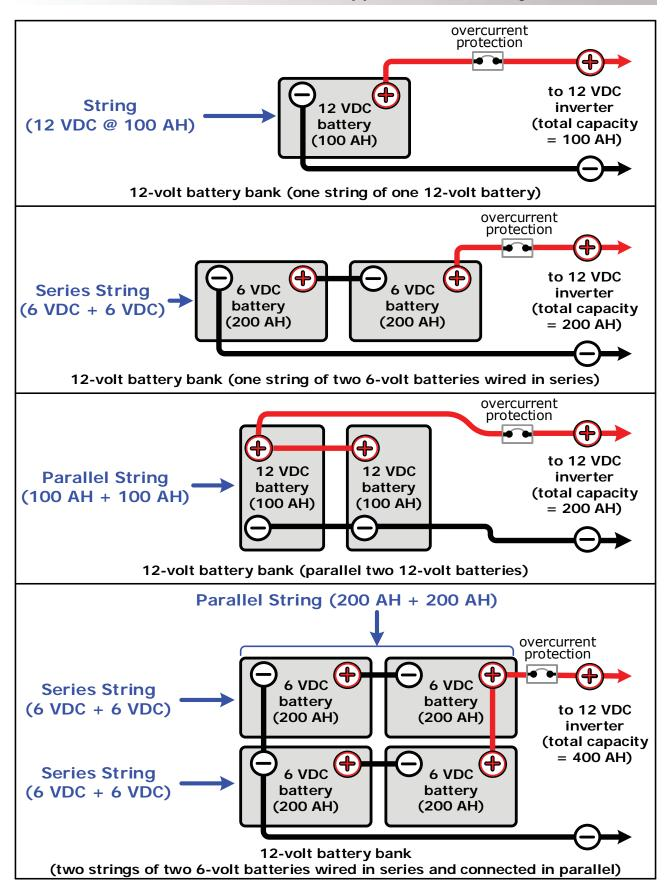
Figure B-4, Battery Bank Wiring Examples (12-volt)
