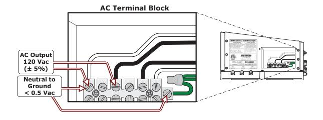
Figure 2-18, AC Voltage Checks
