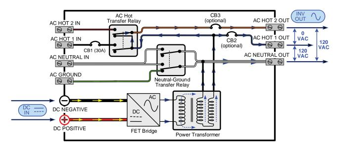
Figure 3-1, Power Flow - Inverter Mode
