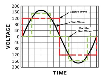
Figure C-1, AC Waveforms
