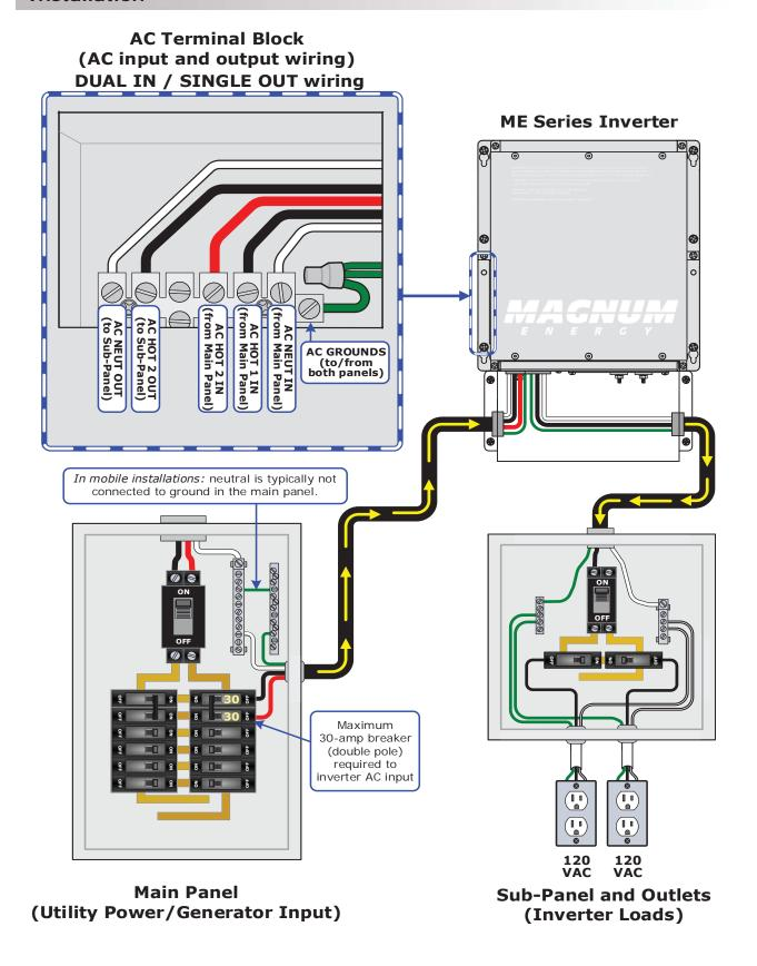
Figure 2-12, AC Wiring for Dual In – Single Out Configurations
