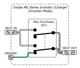
Figure 2-14, Neutral-to-Ground Connection (Inverter Mode)
