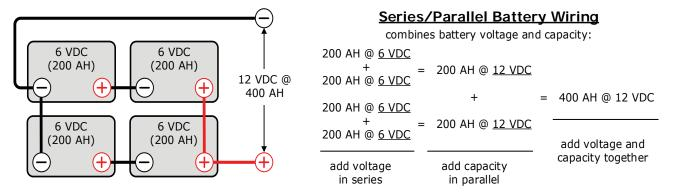
Figure B-3, Series-Parallel Battery Wiring
