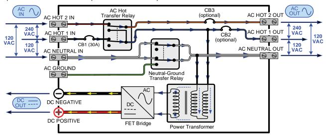
Figure 3-2, Power Flow - Standby Mode
