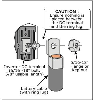
Figure 2-6, Inverter DC Hardware Installation
