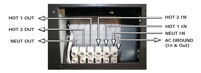
Figure 2-8, AC Terminal Block
