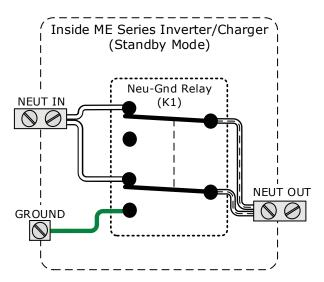
Figure 2-15, Neutral-to-Ground Connection (Standby Mode)
