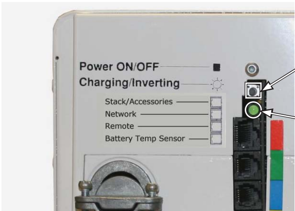
Figure 4-1, Performing an Inverter Reset
