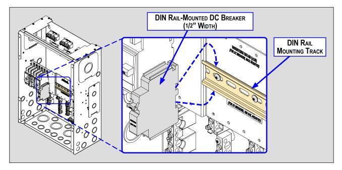
Figure A6-1, Installing DIN Rail-Mounted DC Breakers
