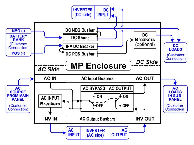
Figure 5-1, MP Functional Diagram
