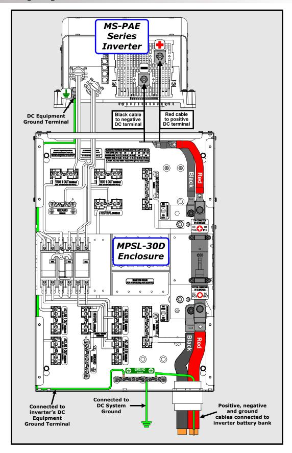
Figure 4-3c, MPSL-30D DC Wiring
