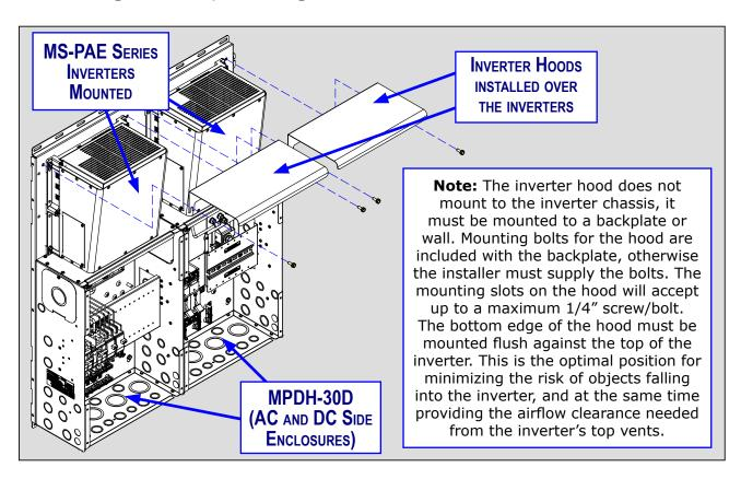
Figure 3-16f, Mounting the Inverter Hoods - MP Dual Enclosure
