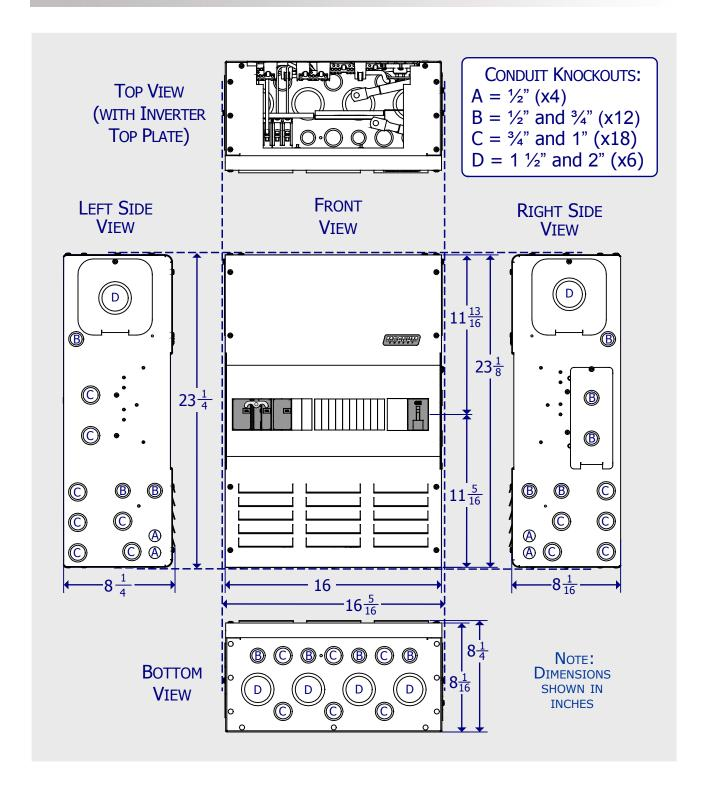
Figure 3-13, MPSL/MPSH Dimensions and Knockout Location/Sizes
