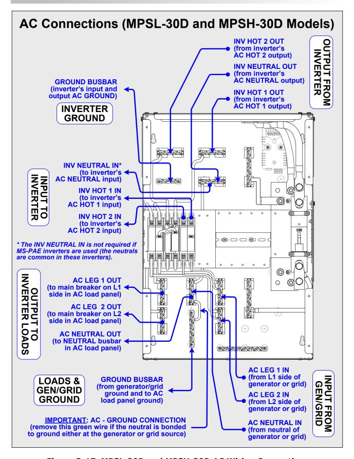
Figure 3-17, MPSL-30D and MPSH-30D AC Wiring Connections
