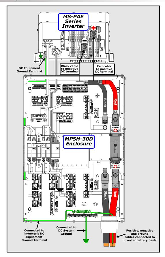
Figure 4-5c, MPSH-30D DC Wiring
