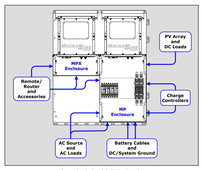
Figure 3-10, Conduit/Wire Routing
