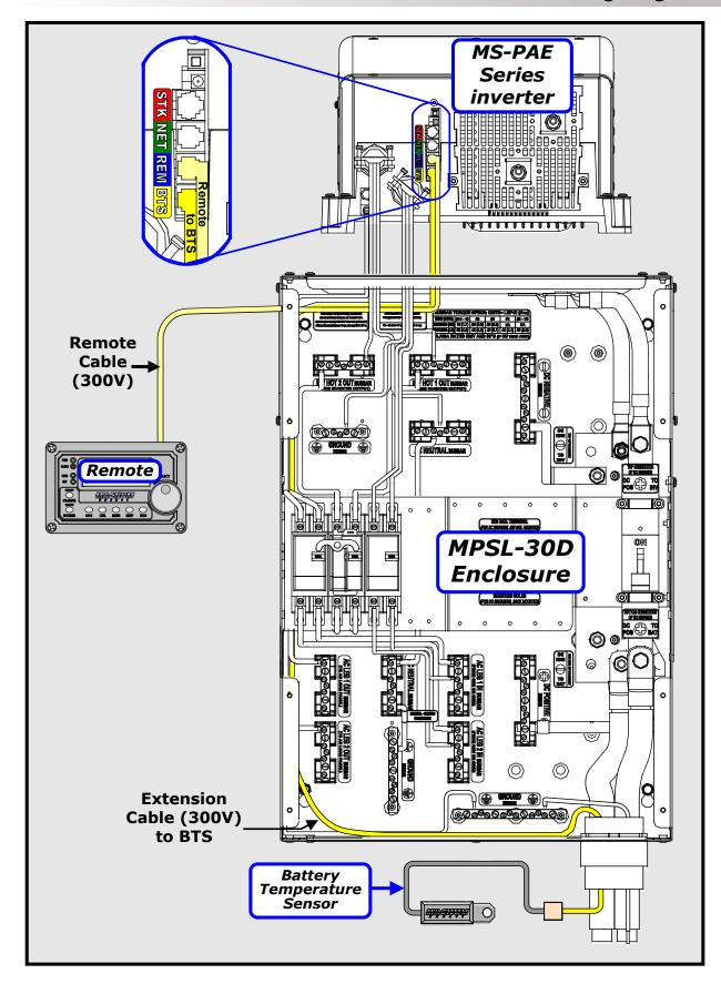
Figure 4-3d, MPSL-30D Communications Wiring
