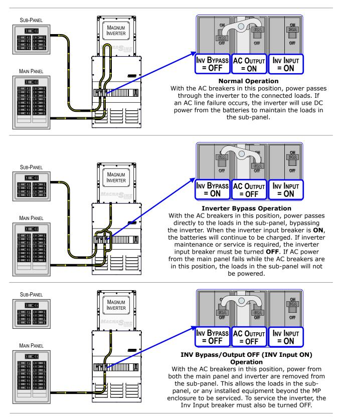
**Note:** The Inverter Input Breaker shown in this figure is a double-pole 30A breaker. On MPSL-60S models this breaker is a single-pole 60A breaker, however the operation of this breaker is the same as shown.
