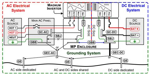
Figure 3-30, Grounding System for Inverter with MP Enclosure
