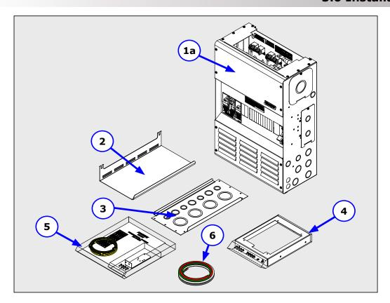
Figure 3-1, Parts Included - MPSL and MPSH Models
