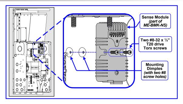
Figure A2-3, Mounting the Sense Module
