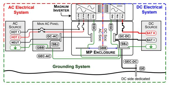
Figure 3-31, Single Connection to DC Ground Rod (Method 1)
