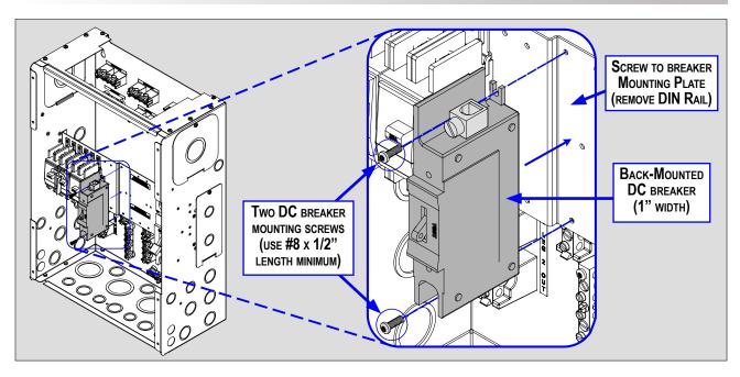
Figure A6-2, Installing Back-Mounted DC Breakers
