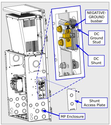
Step 1, Remove Plate and Locate NEG-GND Busbar
