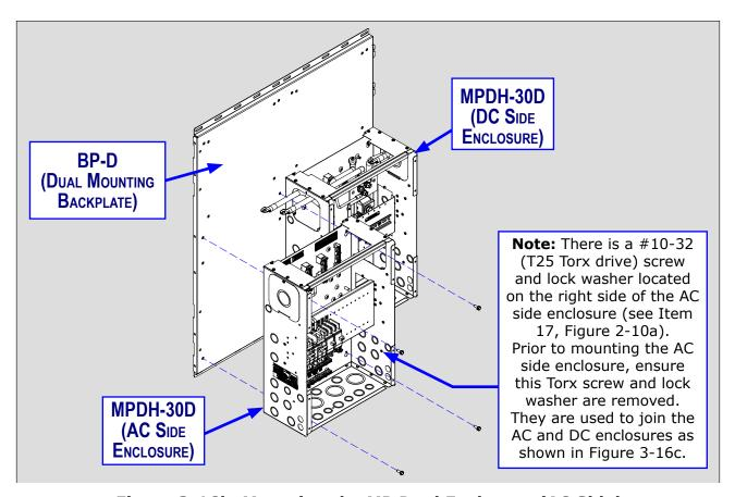
Figure 3-16b, Mounting the MP Dual Enclosure (AC Side)
