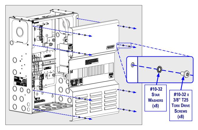
Figure 3-8, Removing Front Cover - Single Enclosure
