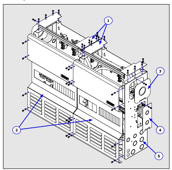
Figure 2-6, MPDH External Components
