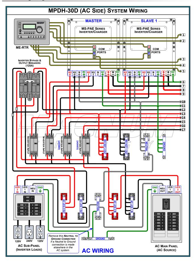
Figure 4-6f.1, MPDH-30D Full System Wiring Diagram (AC Side)
