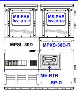
MPSL-30D with **MPXS-30D-R** (MPX - Right Side)
