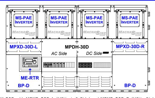
MPDH-30D with MPXD-30D-L (MPX - Left Side) and MPXD-30D-R (MPX - Right Side)
