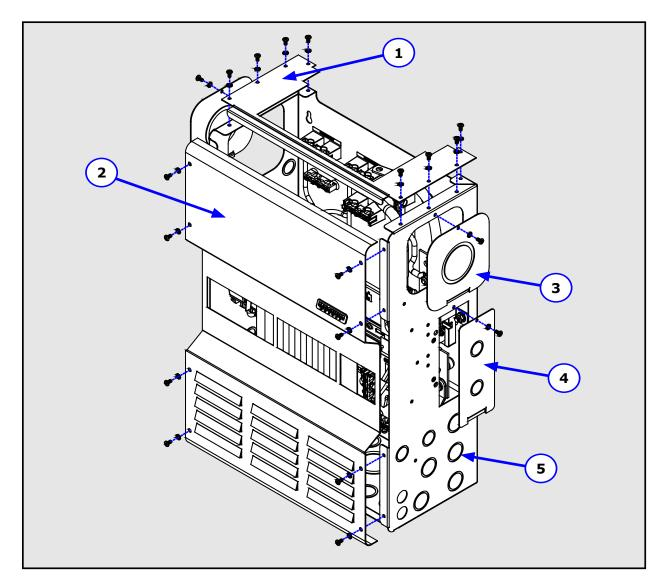
Figure 2-5, MPSL and MPSH External Components
