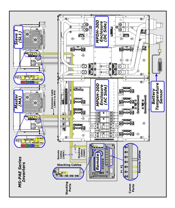
Figure 4-6e, MPDH-30D Communications Wiring
