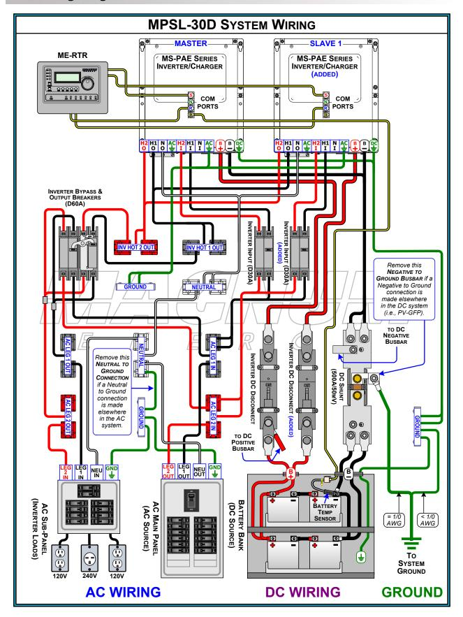
Figure 4-3e, MPSL-30D Full System Wiring Diagram
