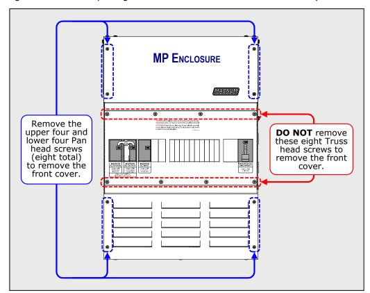
Figure 3-7, Front Cover Screws to Remove
