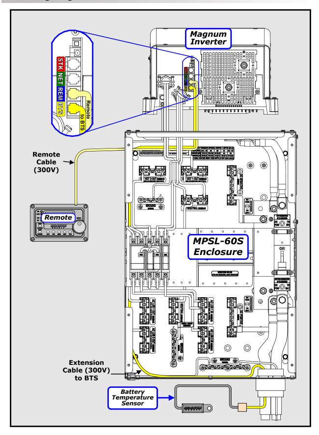
Figure 4-4d, MPSL-60S Communications Wiring
