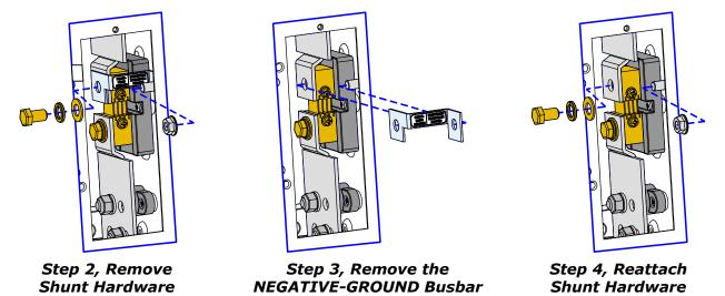
Figure 3-29, Removing the NEGATIVE-GROUND Busbar
