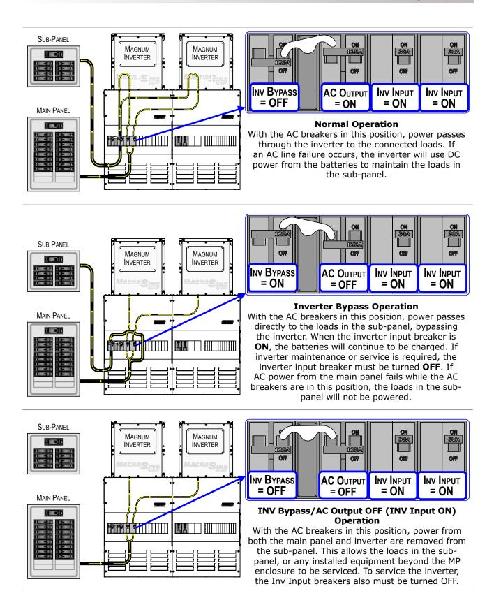
Figure 5-3, 125A Bypass Switch Operation (MPSH-30D and MPDH-30D)
