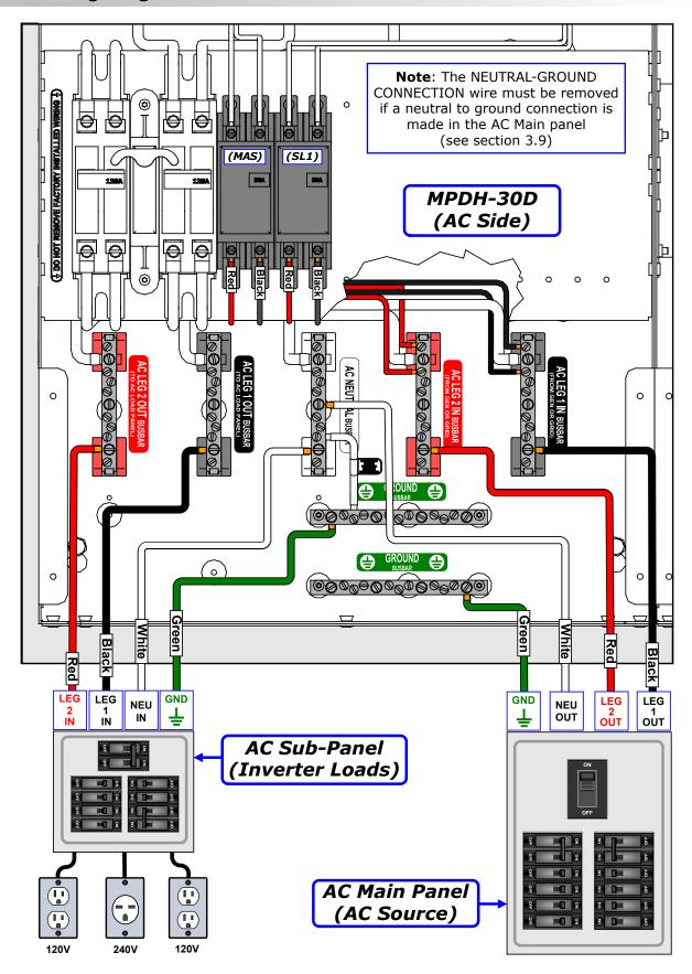
Figure 4-6b, MPDH-30D External AC Wiring
