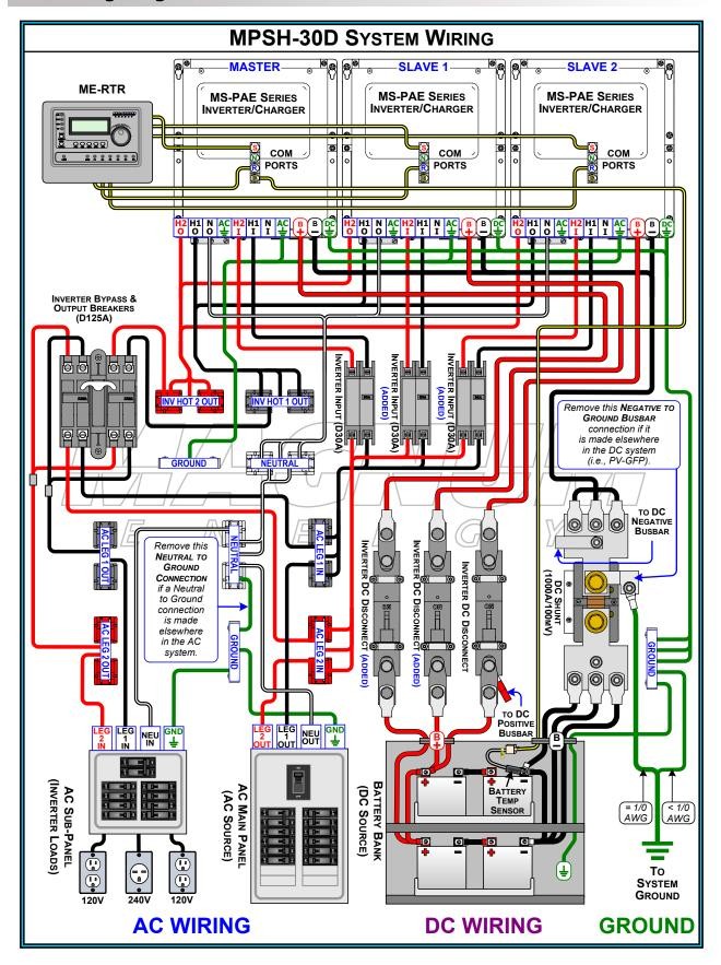
Figure 4-5e, MPSH-30D Full System Wiring Diagram
