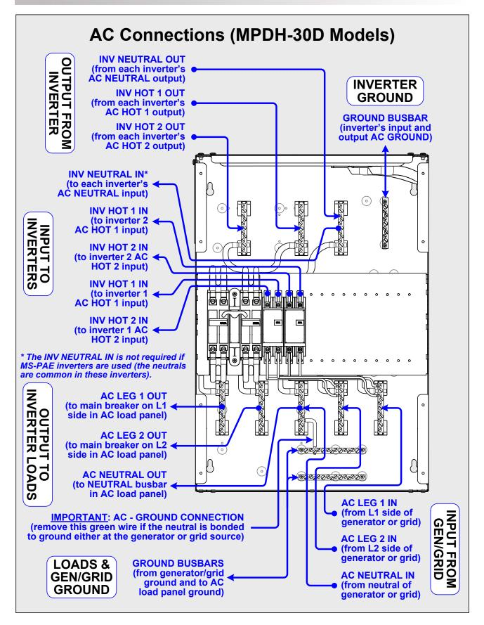
Figure 3-19, MPDH-30D AC Wiring Connections
