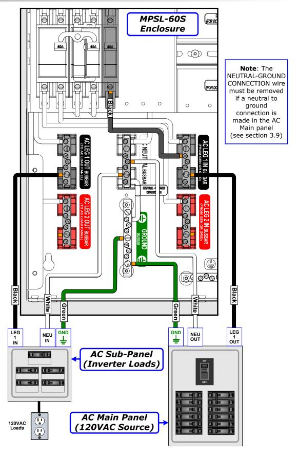
Figure 4-4b, MPSL-60S External AC Wiring
