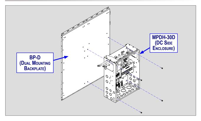
Figure 3-16a, Mounting the MP Dual Enclosure (DC Side)
