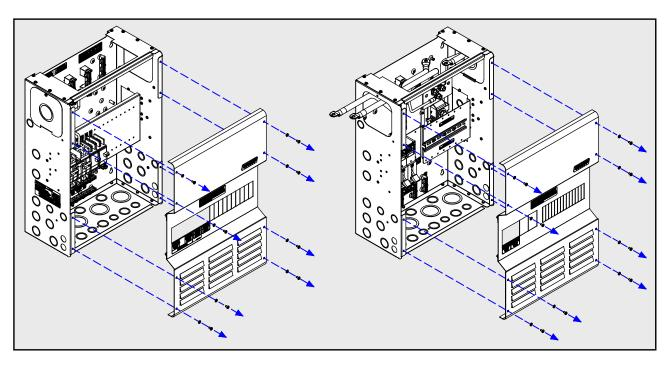
Figure 3-9, Removing Front Covers - Dual Enclosure
