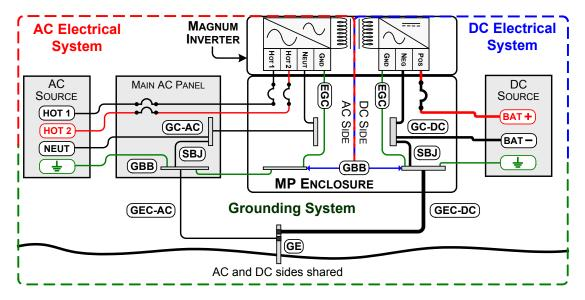
Figure 3-32, Multiple Connections to DC Ground Rod (Method 2)
