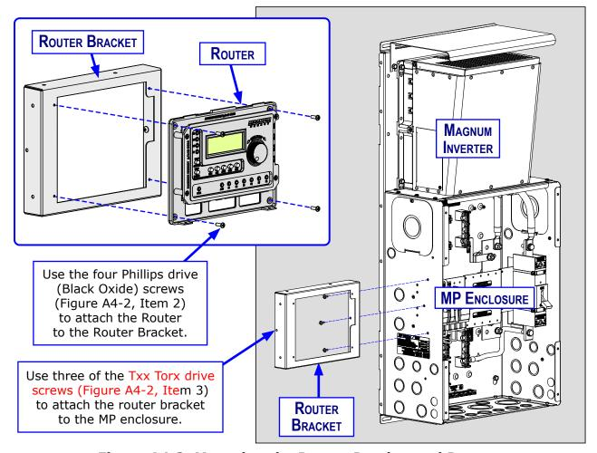
Figure A4-3, Mounting the Router Bracket and Router
