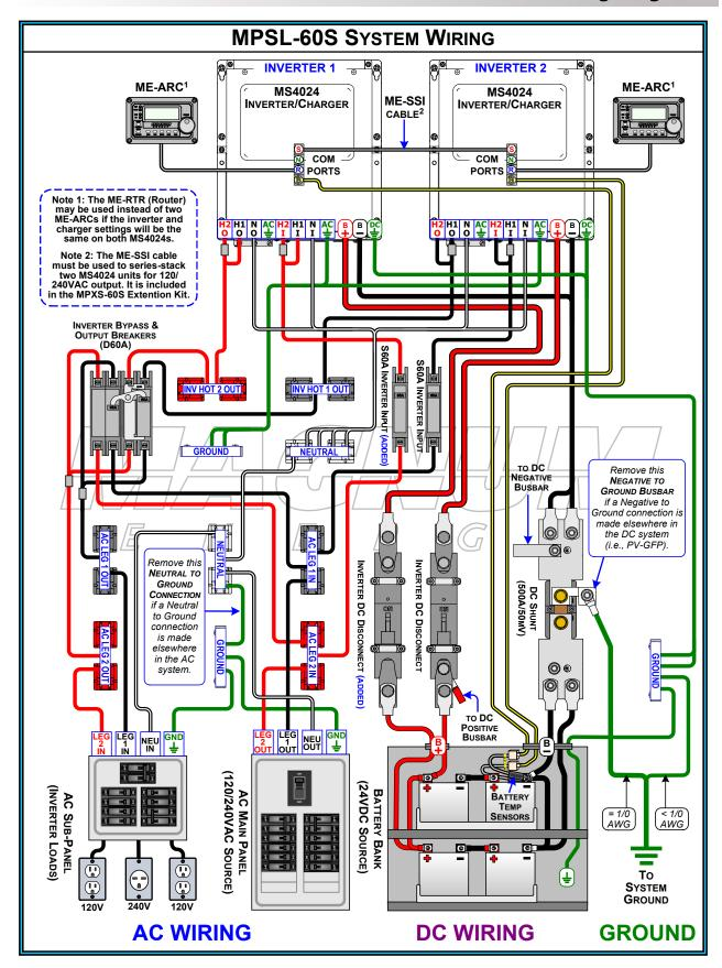
Figure 4-4e, MPSL-60S Full System Wiring Diagram
