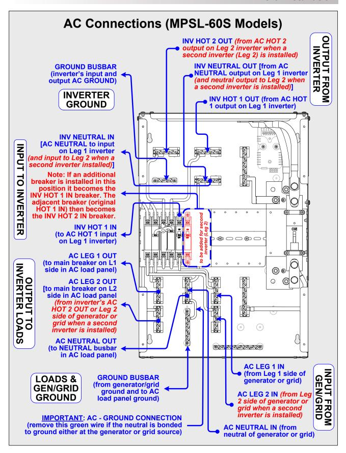
Figure 3-18, MPSL-60S AC Wiring Connections
