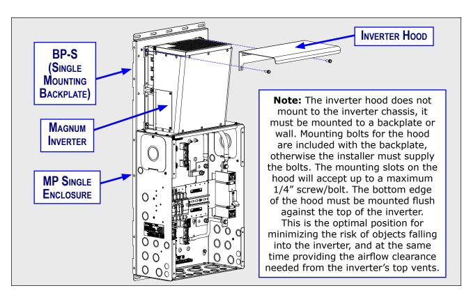
Figure 3-15c, Mounting Inverter Hood - MP Single Enclosure
