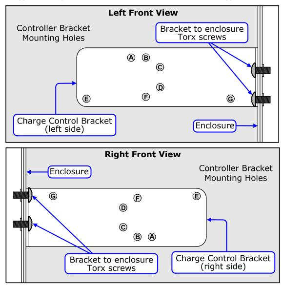
Figure A1-2, Charge Controller Bracket Mounting Holes
