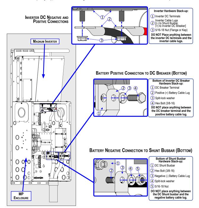
Figure 3-20, DC Hardware Connections
