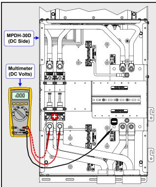
Figure 3-35, DC Voltage Checks - Dual Enclosures (DC Side)
