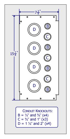
Figure A5-2, Knockout Plate Dimensions and Knockouts
