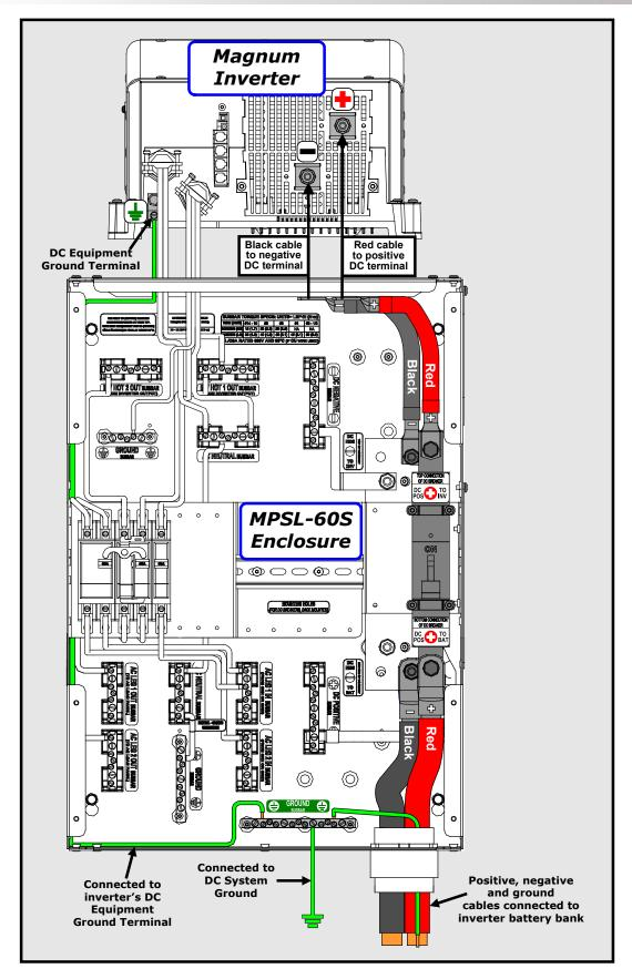
Figure 4-4c, MPSL-60S DC Wiring
