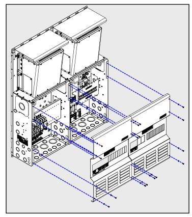
Figure 3-39, Attaching Front Cover - MPSL/MPSH Models
