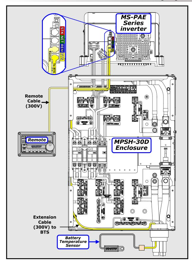
Figure 4-5d, MPSH-30D Communications Wiring
