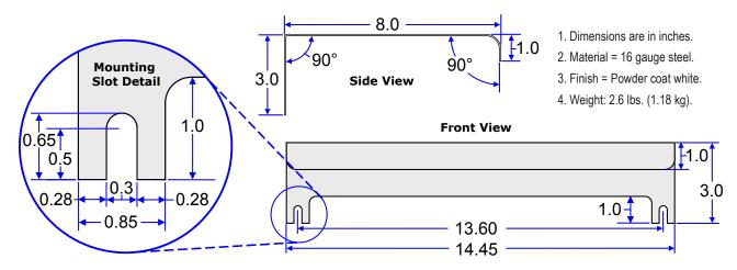
Figure A3-1, Inverter Hood Dimensions
