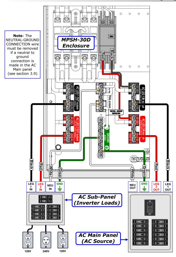
Figure 4-5b, MPSH-30D External AC Wiring
