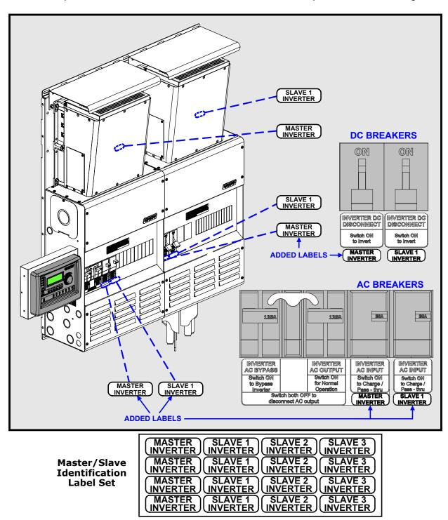
Figure 3-41, Applying Master/Slave Identification Labels
