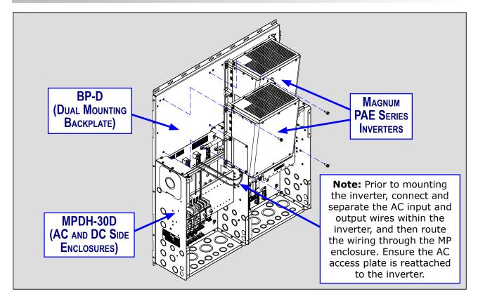
Figure 3-16e, Mounting Second Inverter - MP Dual Enclosure
