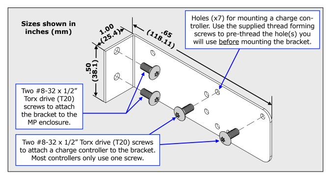
Figure A1-1, Charge Controller Bracket - Physical Dimensions
