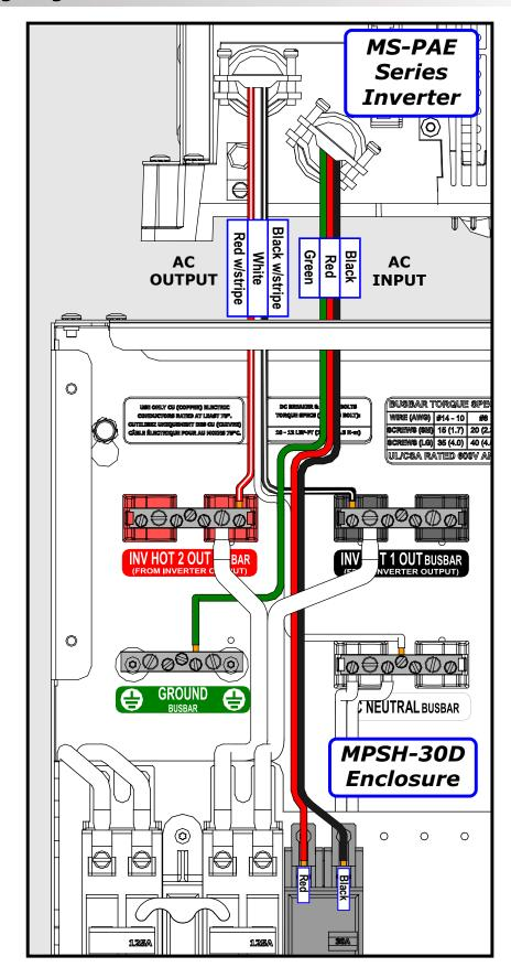
Figure 4-5a, MPSH-30D Inverter AC Wiring
