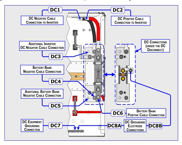
Figure 3-21, DC Wiring Connection Points for MPSL Models
