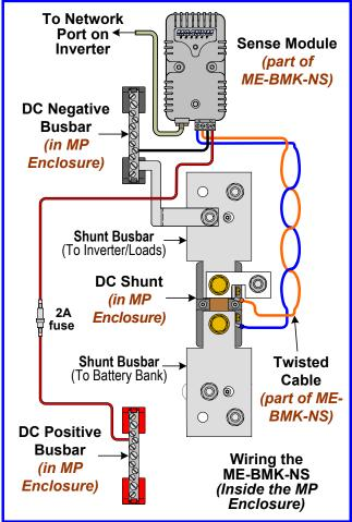
Figure A2-1, Accessing the DC Shunt
