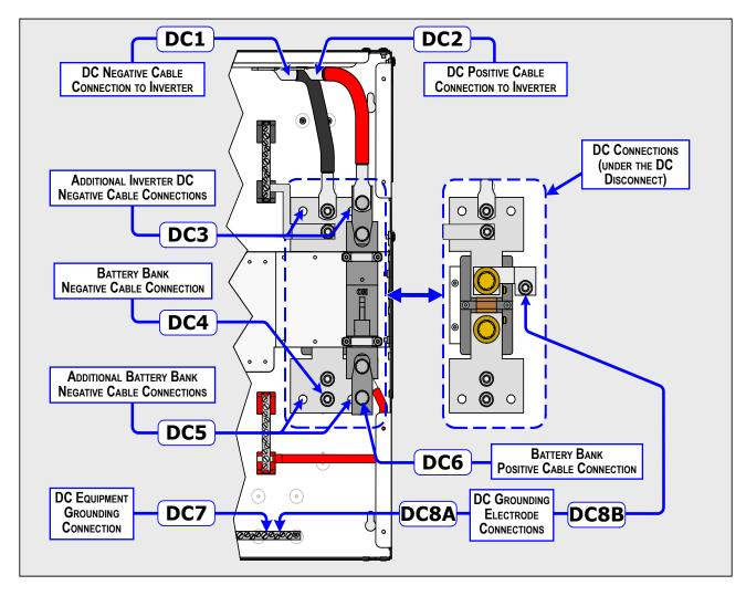
Figure 3-22, DC Wiring Connection Points for MPSH-30D
