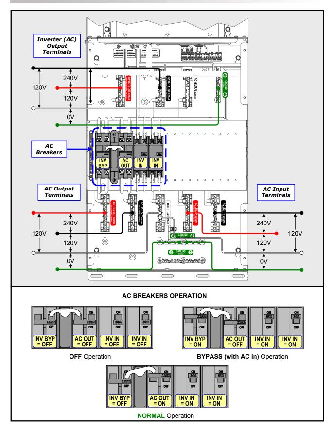
Figure 3-38, AC Voltage Checks - MPDH-30D (AC Side) Models
