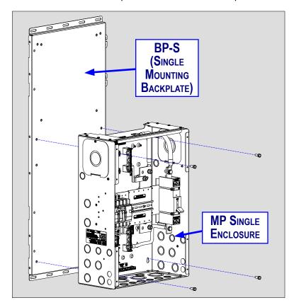
Figure 3-15a, Mounting the MP Single Enclosure
