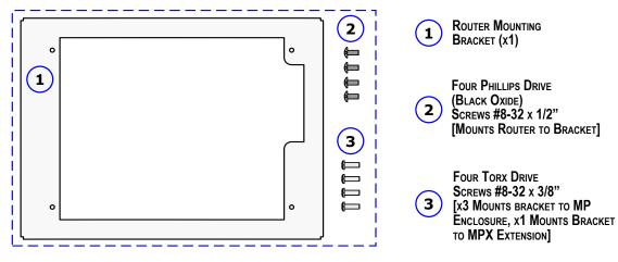
Figure A4-2, Router Bracket Kit
