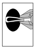
Figure 3-11, Removing Knockouts
