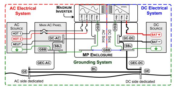
Figure 3-33, Multiple Connections to DC Ground Rod (Method 3)
