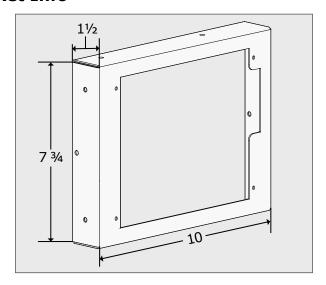
Figure A4-1, Router Bracket Dimensions
