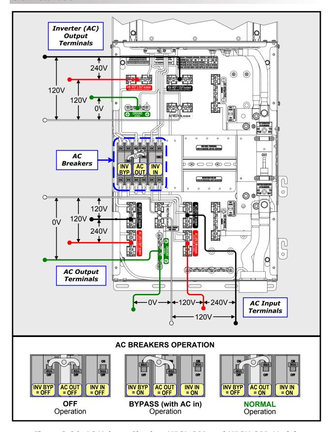
Figure 3-36, AC Voltage Checks - MPSL-30D and MPSH-30D Models
