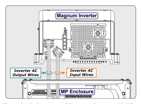
Figure 3-12, Connect and Separate Inverter AC Wires
