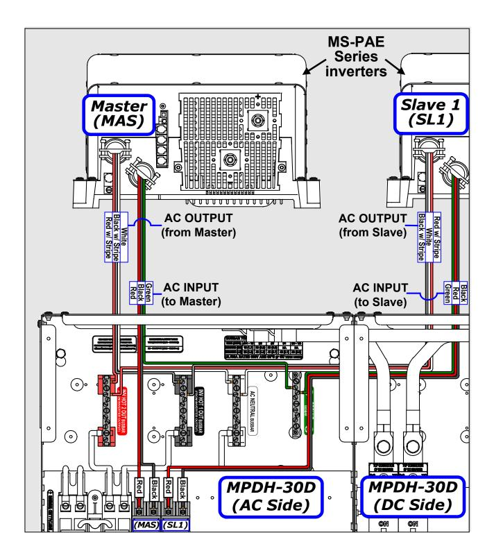
Figure 4-6a, MPDH-30D Inverter AC Wiring
