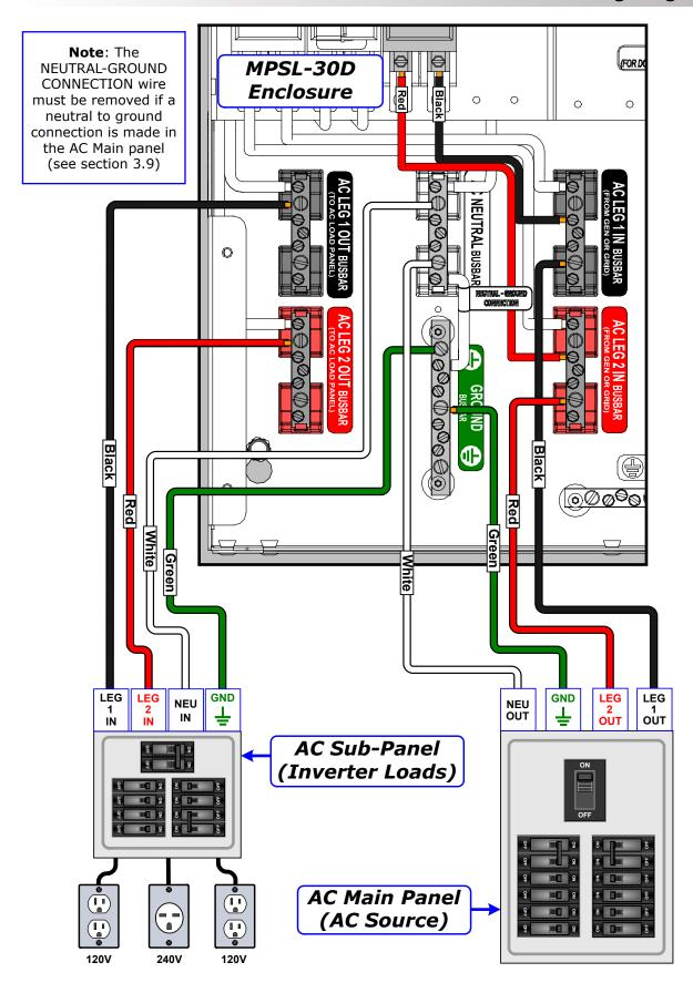
Figure 4-3b, MPSL-30D External AC Wiring
