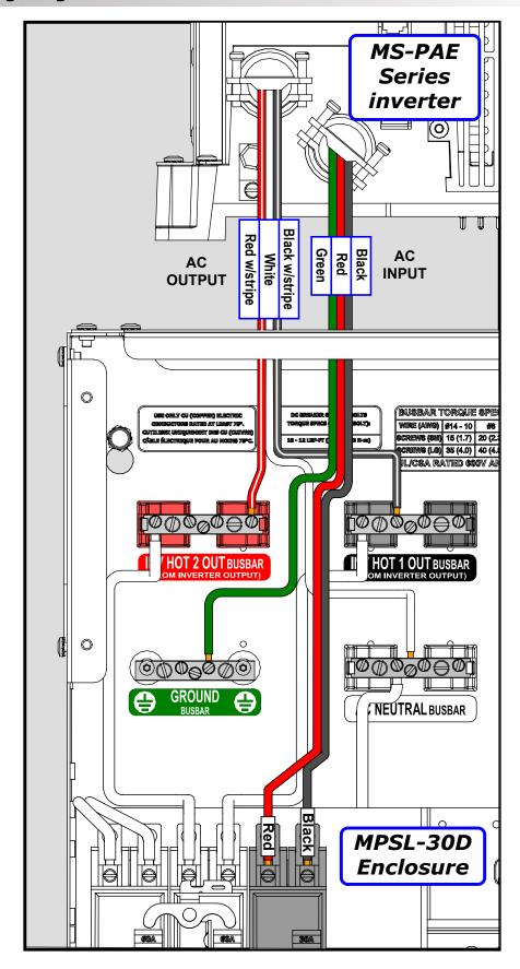
Figure 4-3a, MPSL-30D Inverter AC Wiring
