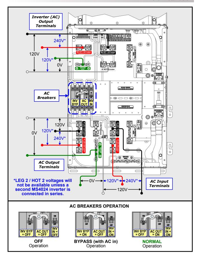
Figure 3-37, AC Voltage Checks - MPSL-60S Models
