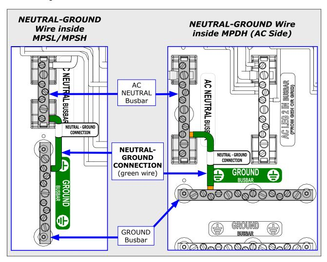
Figure 3-28, Removing the NEUTRAL-GROUND Wire
