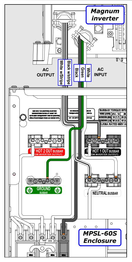
Note: This figure shows wiring inside the MPSL-60S. for one MS4024 - as LEG 1 (120V AC only).
