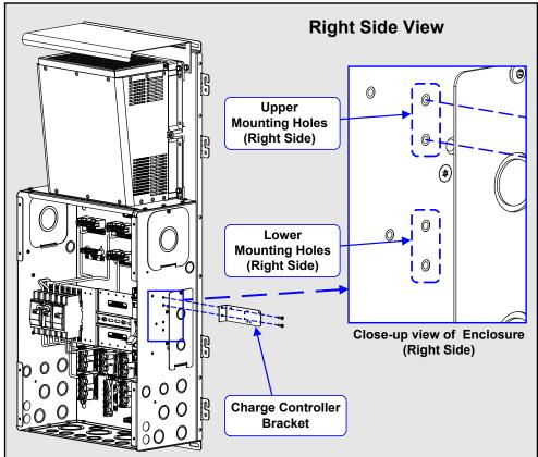
Figure A1-3, Holes Used to Mount Bracket on MP Enclosure
