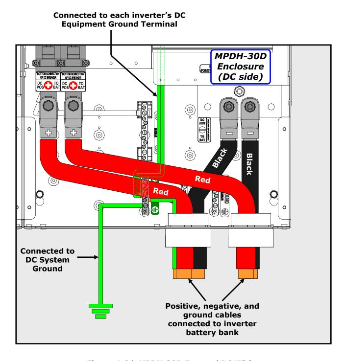
Figure 4-6d, MPDH-30D External DC Wiring
