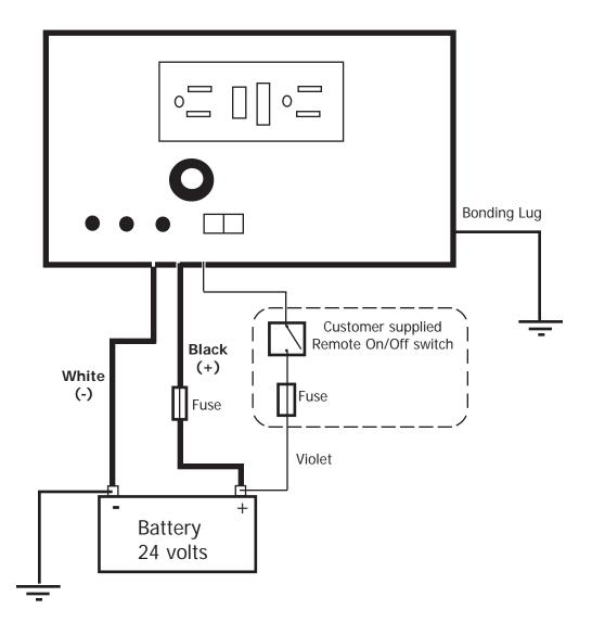
**NOTE:** The Inverter must be connected to the 24 Volt battery bank with the correct polarity. The black wire is "POSITIVE (+)", and the white wire is "NEGATIVE (-)". Connecting the inverter improperly will cause damage that is not covered under the warranty.
