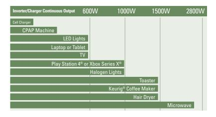
The pure sine wave MS2812 Inverter/Charger is ideal when a microwave will be used.
