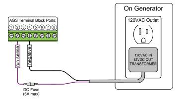
Option 3 – Use an external 120 VAC coiled relay to bring the generator's battery voltage to the AGS run sense port (AGS Terminal Block Port #2) only while the generator is running. The generator's battery voltage must be 10-40 VDC.
