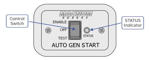
Figure 4-2, Remote Switch Controls and Indicators
