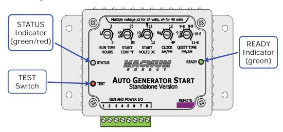
Figure 4-1, Controller Front Panel Controls and Indicators
