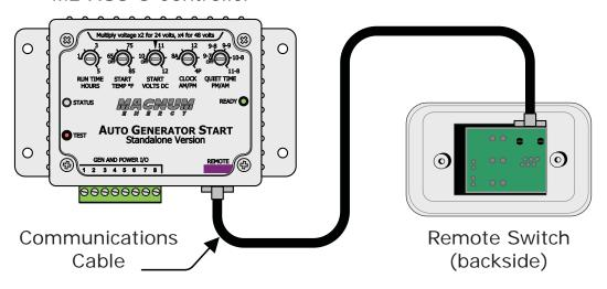
Figure 2-4, Communication Cable Connection
