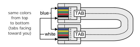
Figure 2-5, Communication Cable (Data Type)
