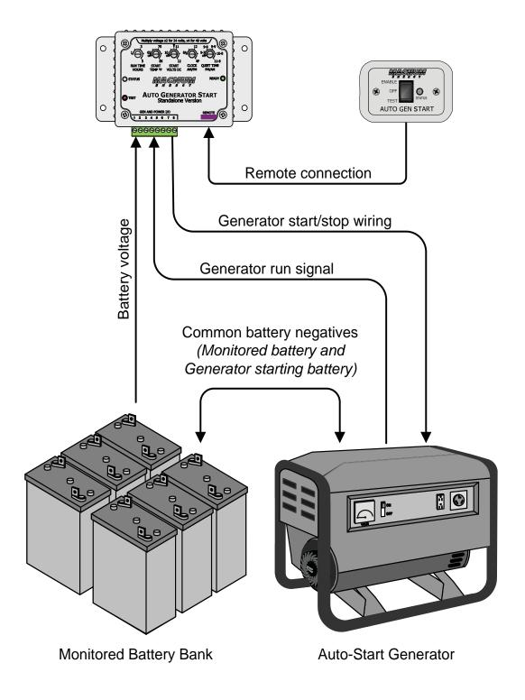
Figure 2-1, ME-AGS-S System Diagram
