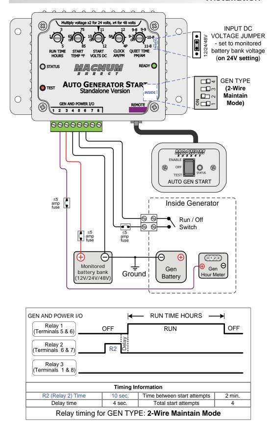
Figure 2-9, Two-wire Start Type Generators
