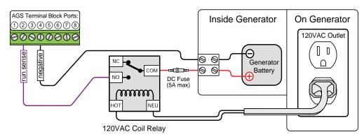
Figure 2-6, Generator Run Sense Options
