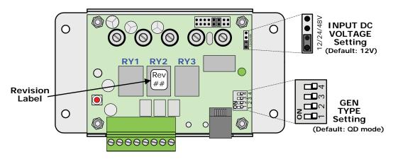
Figure 3-1, Inside the AGS Controller
