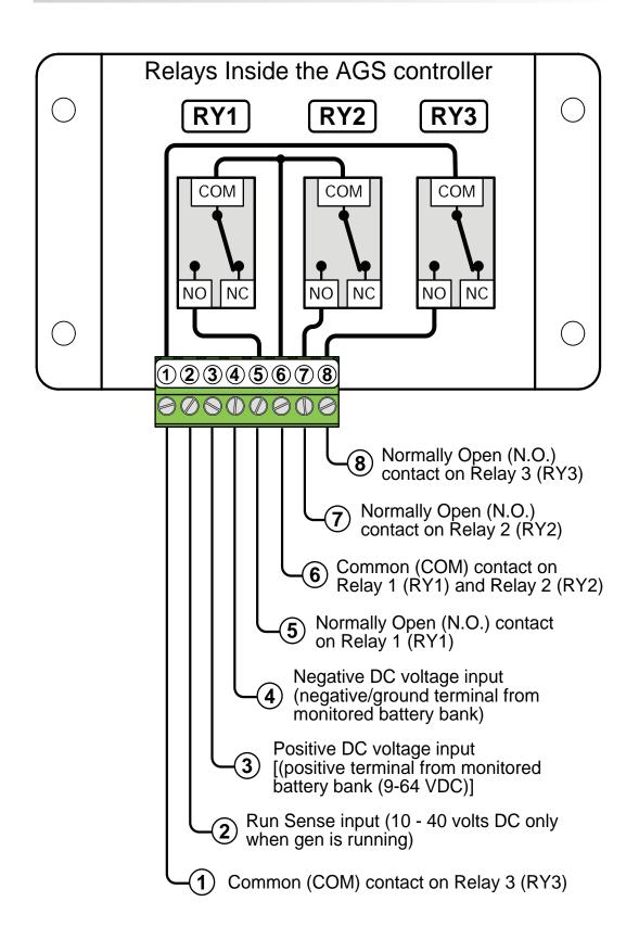
Figure 2-7, Wiring to the AGS Controller's Terminal Block
