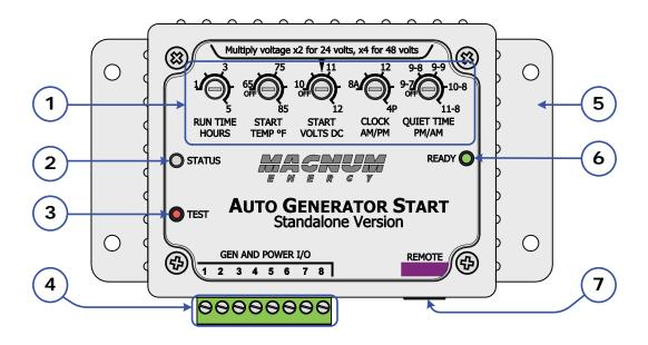
Figure 1-3, ME-AGS-S Controller Features
