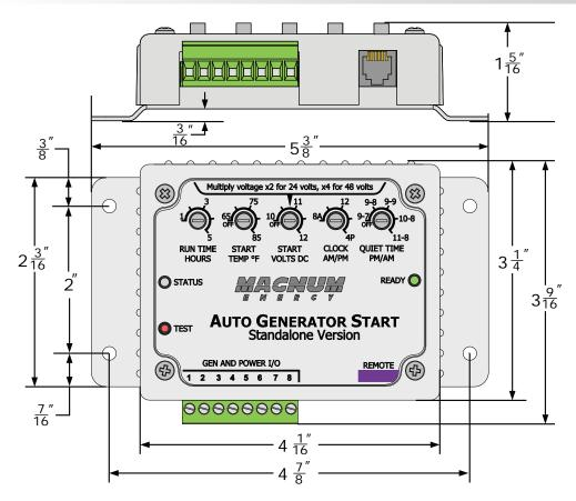
Figure 2-2, Controller Dimensions
