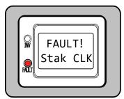
**Stak CLK** appears on the LCD and the FAULT (red) LED is on. The INV (green) LED is off.
