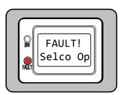
**Selco Op** appears on the LCD and the FAULT (red) LED is on. The INV (green) LED is off.
