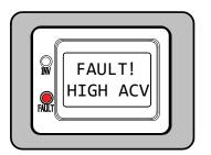
**HIGH ACV** appears on the LCD and the FAULT (red) LED is on. The INV (green) LED is off.
