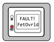
**FetOvrld** appears on the LCD and the FAULT (red) LED is on. The INV (green) LED is off.
