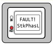
**StkPhasL** appears on the LCD and the FAULT (red) LED is on. The INV (green) LED is off.
