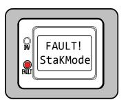
**StaKMode** appears on the LCD and the FAULT (red) LED is on. The INV (green) LED is off.
