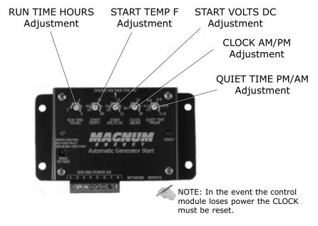
Figure 6 - AGS Controller Adjustments
