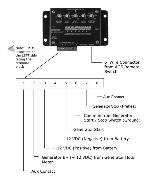
Figure 5 - AGS Connector Pin Legend (from left to right)
