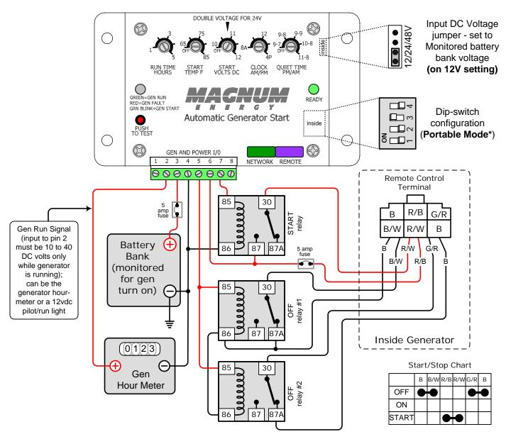
Relays used are SPDT, 30 Amp, 12 VDC coil relays [shown in the non-energized (N.C.) position]
