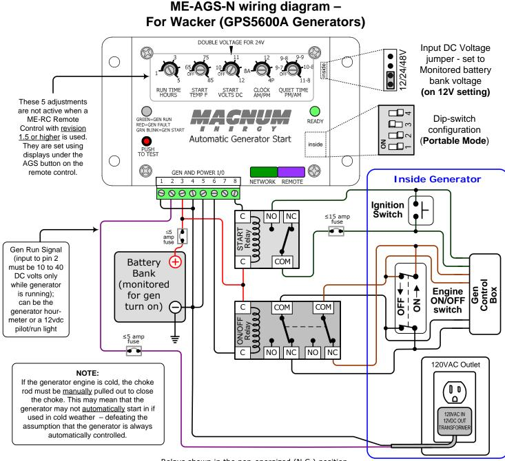
Relays shown in the non-energized (N.C.) position. The START relays is a SPDT ≥15 Amp, 12 VDC coil relays. The ON/OFF relay is a DPDT ≥5 amp, 12 VDC coil relay.
