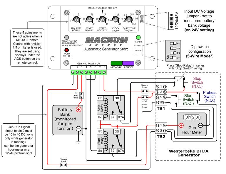
Relays used are SPDT 30 Amp, 12 VDC coil relays [shown in the non-energized (N.C.) position]; popular in automotive sound and security installations. Equivalent to Bosch #0 332 209 150. Mfg. #V23234-A1001-X036.
