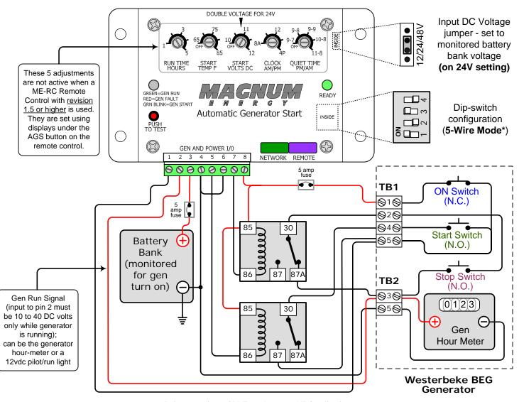
Relays used are SPDT 30 Amp, 12 VDC coil relays [shown in the non-energized (N.C.) position]
