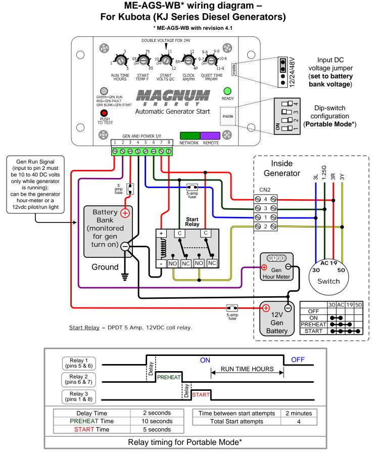
\* to enable Portable Mode, the ME-AGS-WB must be revision 4.1 or higher
