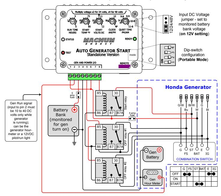
Relays used are SPDT 30 Amp, 12 VDC coil relays [shown in the non-energized (N.C.) position]
