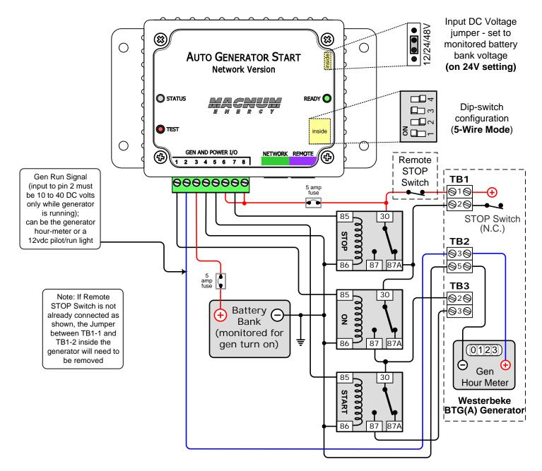
Relays used are SPDT 30 Amp, 12 VDC coil relay; popular in automotive sound and security installations. Equivalent to Bosch #0 332 209 150 or TYCO #V23234-A1001-X036.
