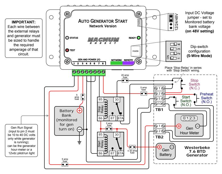
Relays used are SPDT 30 Amp, 12 VDC coil relay; popular in automotive sound and security installations. Equivalent to Bosch #0 332 209 150 or TYCO #V23234-A1001-X036.
