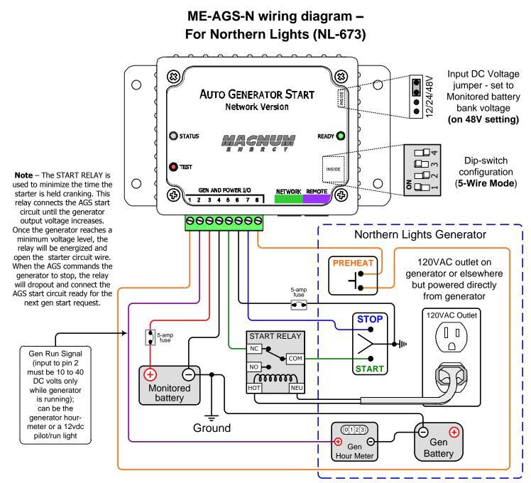
For the START RELAY, use a VOLTAGE MONITOR RELAY that has over/under voltage set-points. This is to adjust the relay to prevent it from energizing until the generator output level is stable enough to power a load. Examples are: **VMKP120A** (www.macromatic.com) or **CSJ-38-70010** (www.tycoelectronics.com)
