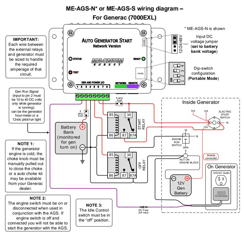
START and OFF Relays = SPDT 30 Amp, 12 VDC coil relay; popular in automotive sound and security installations. Equivalent to Bosch #0 332 209 150 or TYCO #V23234-A1001-X036.
