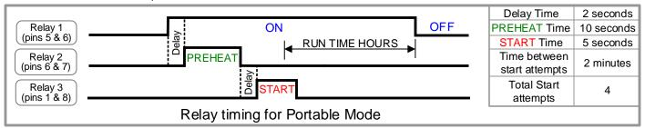
Magnum Energy, Inc. provides this diagram to assist in the installation of the Auto-Generator Start controller. Since the use of this diagram and the conditions or methods of installation, operation and use are beyond the control of Magnum Energy, Inc., we do not assume responsibility and expressly disclaim liability for loss, damage or expense arising out of the installation, operation and use of this unit.
