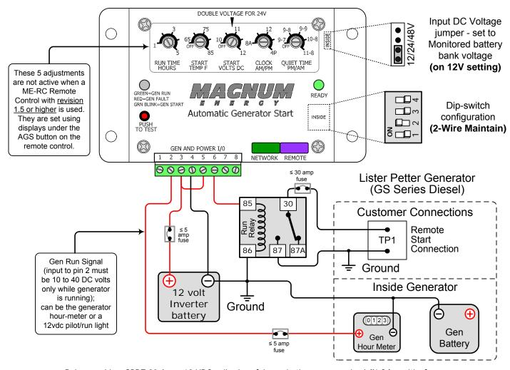
Relay used is a SPDT 30 Amp, 12 VDC coil relays [shown in the non-energized (N.C.) position]; popular in automotive sound and security installations. Equivalent to Bosch #0 332 209 150. Mfg. #V23234-A1001-X036.
