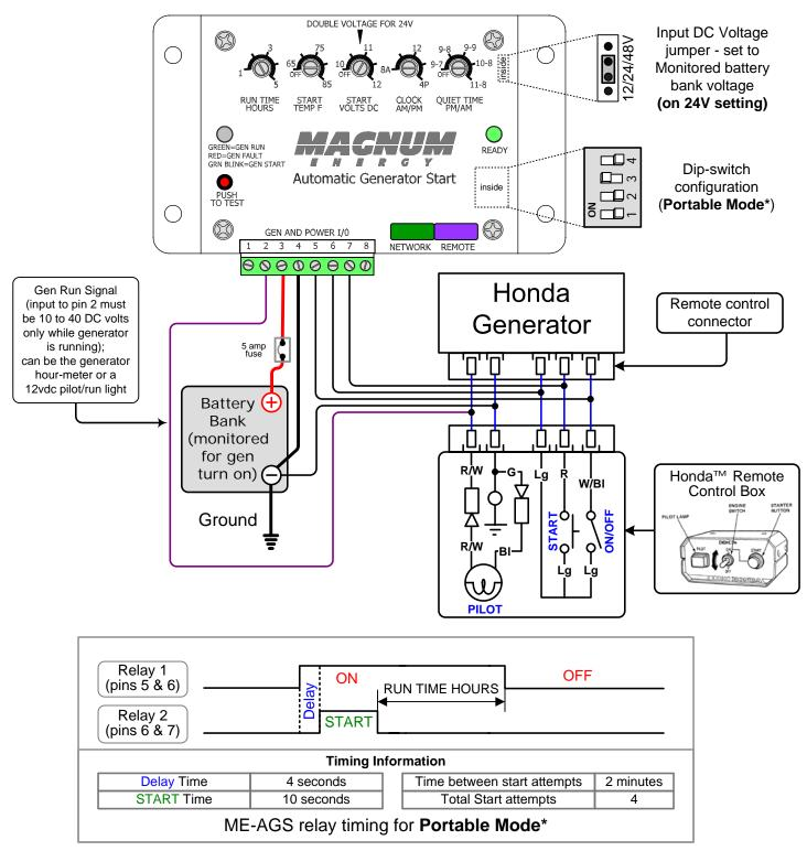
\* to enable Portable Mode, the ME-AGS must be revision 3.2 or higher
