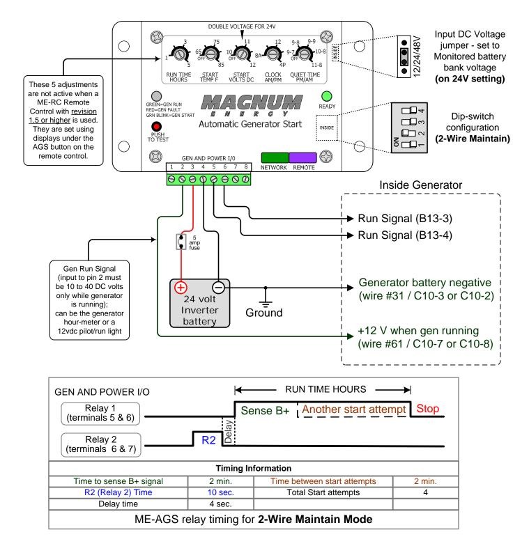
Magnum Energy, Inc. provides this diagram to assist in the installation of the Auto-Generator Start controller. Since the use of this diagram and the conditions or methods of installation, operation and use are beyond the control of Magnum Energy, Inc., we do not assume responsibility and expressly disclaim liability for loss, damage or expense arising out of the installation, operation and use of this unit.
