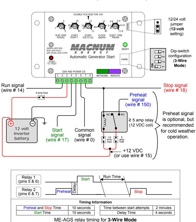
ME-AGS wiring diagram – For Generac Diesel (Quiet Pack Series)
