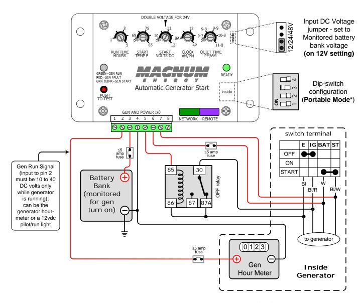
"OFF Relay" is a SPDT 30 Amp, 12 VDC coil relays [shown in the non-energized (N.C.) position]
