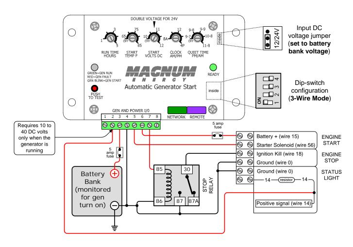
Relay used is a SPDT 30 Amp, 12 VDC coil relays [shown in the non-energized (N.C.) position]
