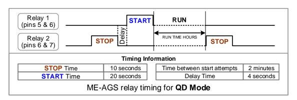
This diagram is provided to assist in the installation of the Auto Generator Start controller. Since the use of this diagram and the conditions or methods of installation, operation and use are beyond the control of Sensata Technologies (Magnum Energy Products), we do not assume responsibility and expressly disclaim liability for loss, damage or expense arising out of the installation, operation and use of this unit.
