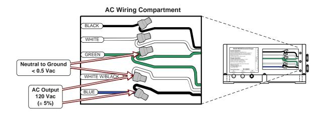
Figure 2-22, AC Voltage Checks (ME2000 model)
