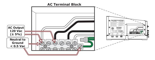
Figure 2-21, AC Voltage Checks (Models with terminal block)
