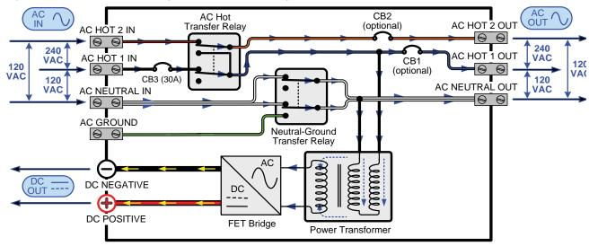
Figure 3-2, Power Flow – Standby Mode
