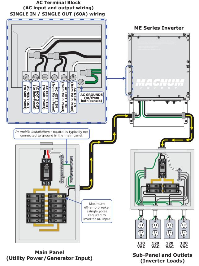
Figure 2-11, AC Wiring for Single In - Single Out (60A) Configurations
