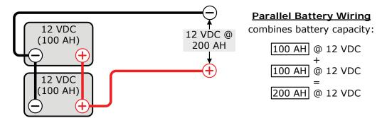
Figure B-2, Parallel Battery Wiring
