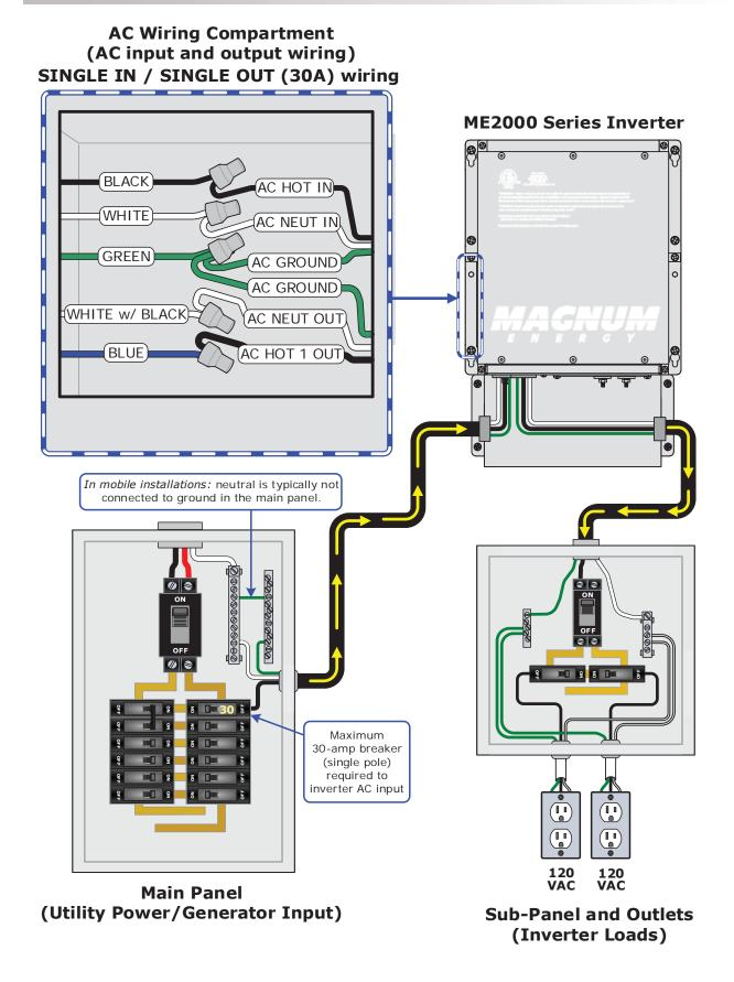
Figure 2-15, AC Wiring for ME2000 Models
