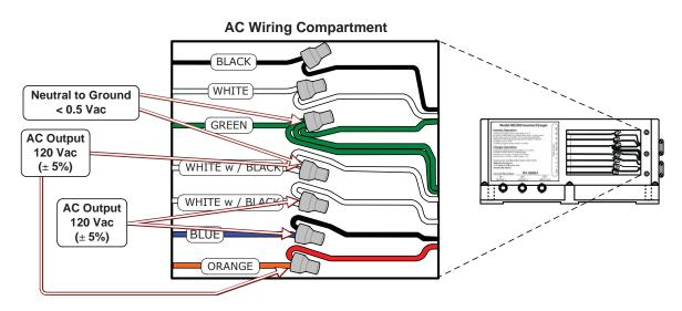
Figure 2-23, AC Voltage Checks (ME2000-15B/-20B models)
