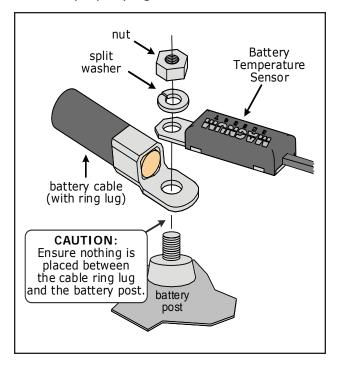
Figure 2-6, Battery Hardware Installation
