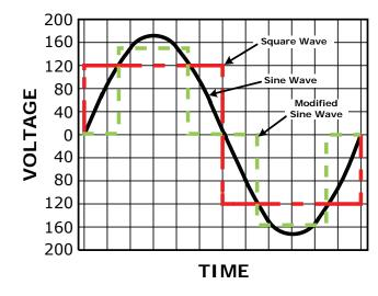
Figure C-1, AC Waveforms
