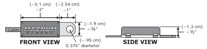
Figure 2-8, Battery Temperature Sensor
