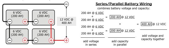
Figure B-3, Series-Parallel Battery Wiring
