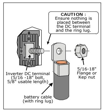
Figure 2-7, Inverter DC Hardware Installation
