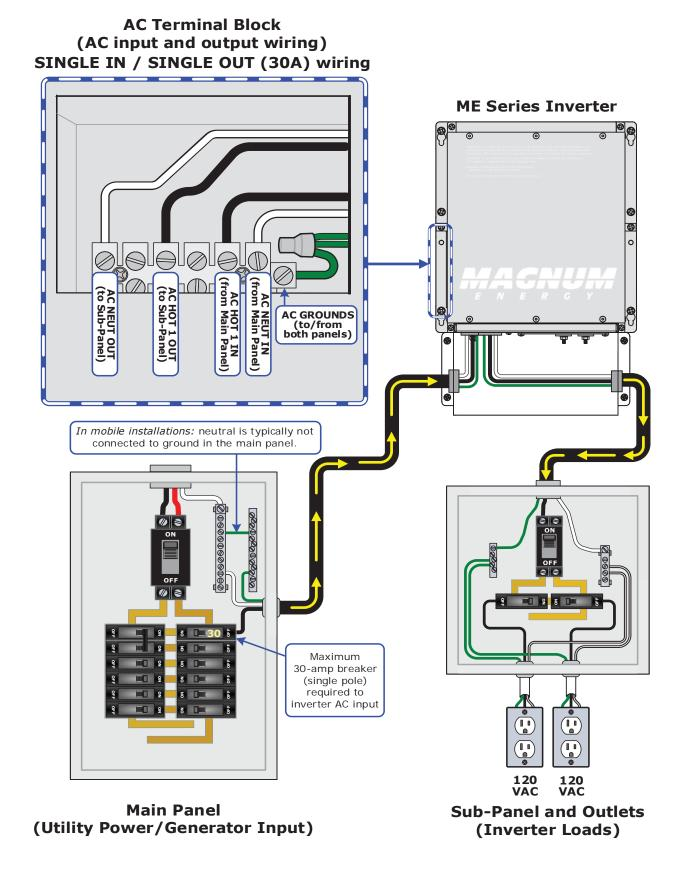
Figure 2-10, AC Wiring for Single In – Single Out (30A) Configurations
