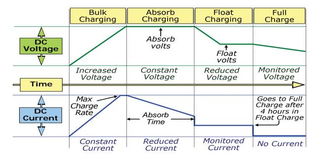
Figure 3-3, Automatic 4-Stage Charging Graph
