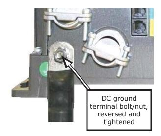
Figure 2-19, Connecting a Large DC Ground Wire
