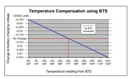
Figure 3-4, BTS Temperature to Charge Voltage Change
