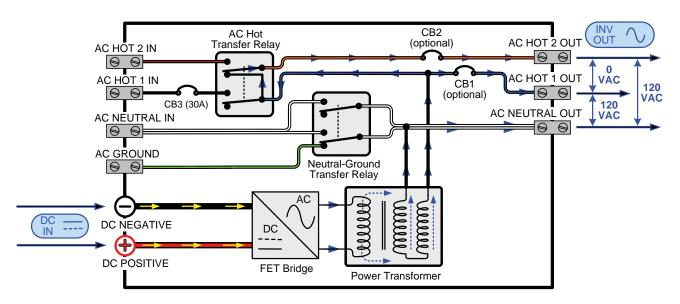
Figure 3-1, Power Flow - Inverter Mode
