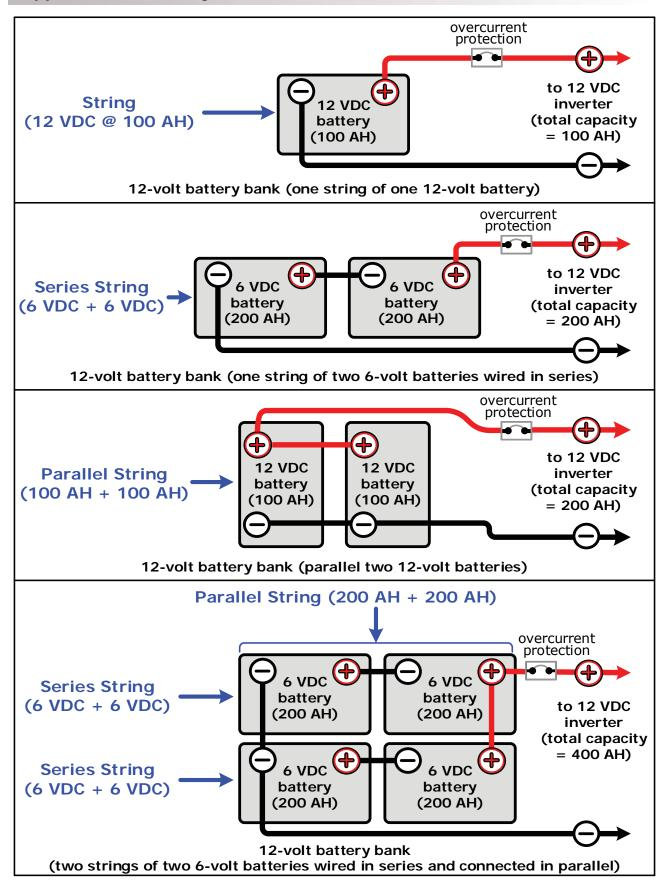
Figure B-4, Battery Bank Wiring Examples (12-volt)
