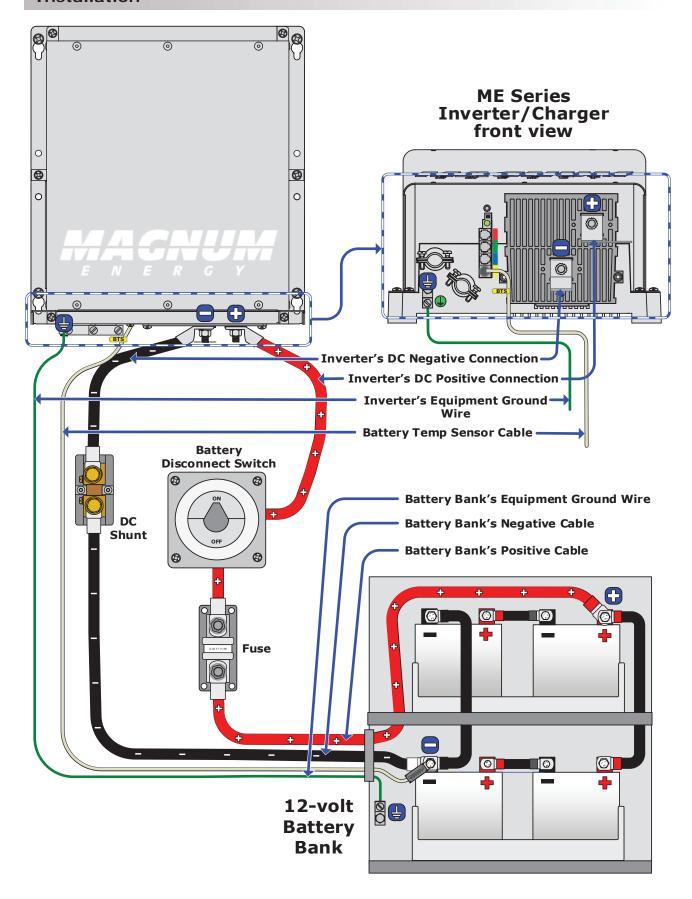
Figure 2-5, DC and Battery Temperature Sensor Wiring
