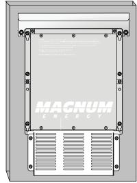
WALL MOUNTED (DC TERMINALS ON THE BOTTOM\*)
