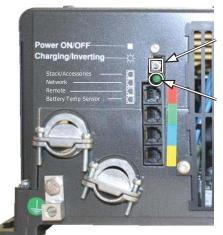
Power ON/OFF pushbutton switch
