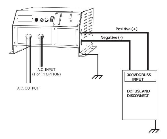
**WARNING:** Connecting the power supply with the wrong polarity to the inverter will cause damage that is not covered under the warranty.
