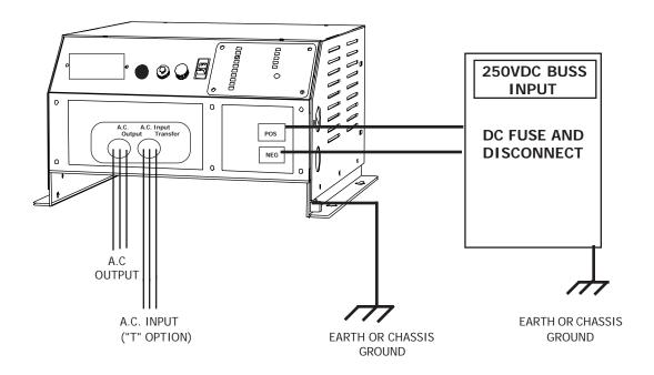
FIG. 1 INSTALLATION WIRING
