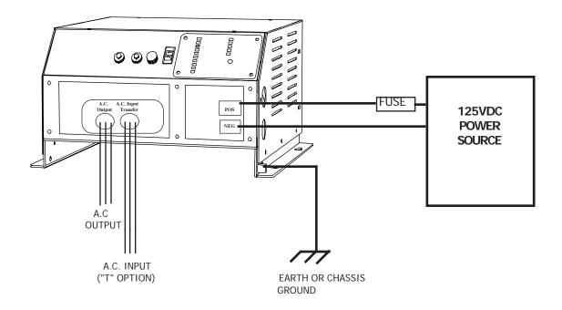
FIG. 1 INSTALLATION WIRING
