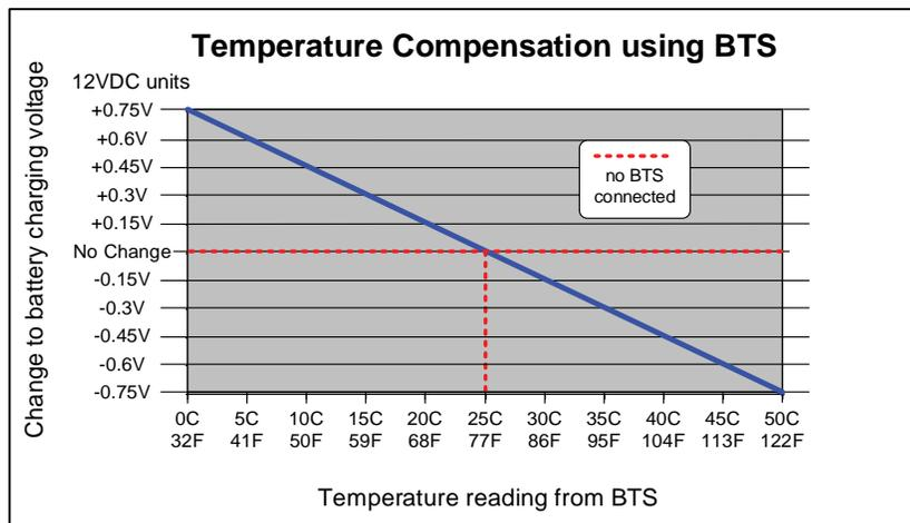
Figure 3-4, BTS Temperature to Charge Voltage Change
