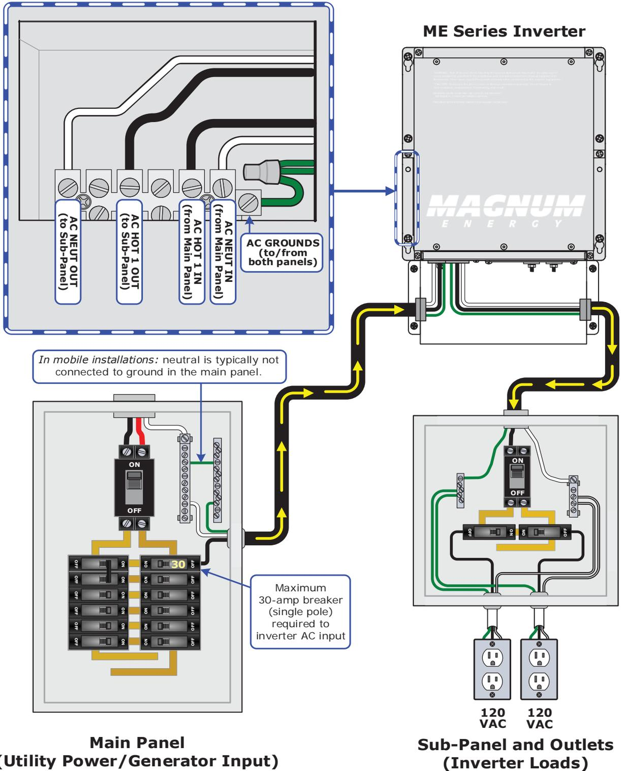
Figure 2-9, AC Wiring for Single In – Single Out (30A) Configurations
