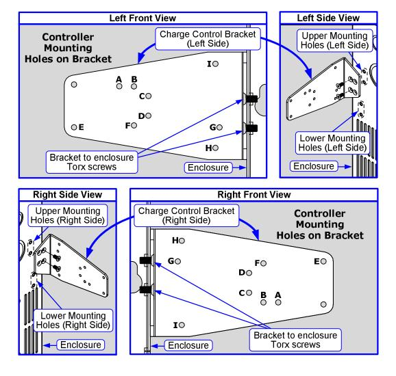
Figure 2, Mounting Holes
