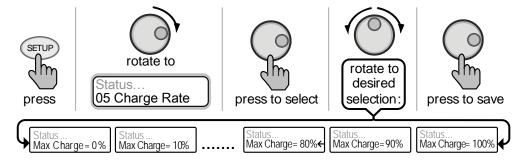
Figure 3-10, SETUP: 05 Charge Rate Selections
