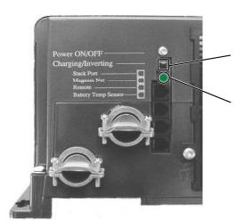
Press and hold the Power ONOFF push-button for 15 seconds
