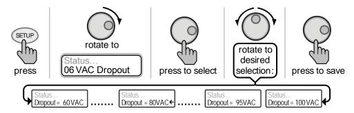
Figure 3-11, SETUP: 06 VAC Dropout Selections
