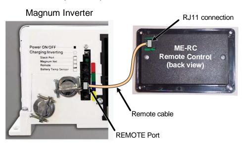
Figure 2-2, Remote Control Connections
