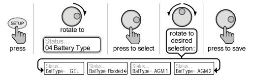
Figure 3-9, SETUP: 04 Battery Type Selections
