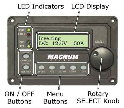
Figure 5-1, ME-RC Front Panel Controls and Indicators
