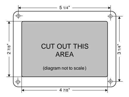
Figure 2-1, Remote Cut-Out Dimensions
