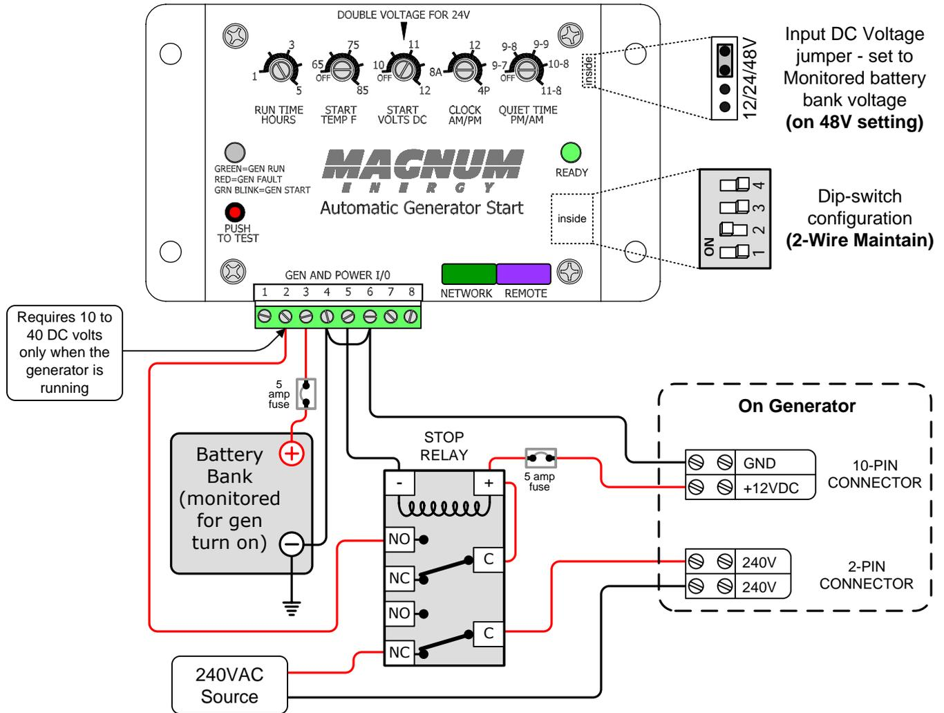
Relay used is a DPDT, 12 VDC coil relay, Contacts rated for 240VAC and 12VDC (≥5 Amps)
