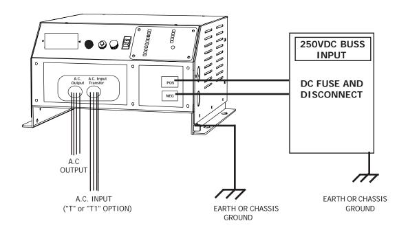
FIG. 1 INSTALLATION WIRING
