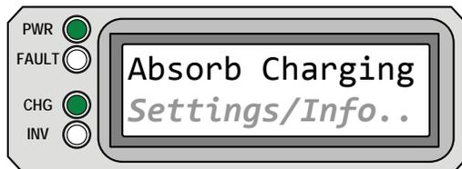
**Absorb Charging** appears on LCD; PWR (green) is on solid and CHG (green) LED is typically on solid, but may blink. FAULT (red) LED is off. INV (green) LED could be on or off.
