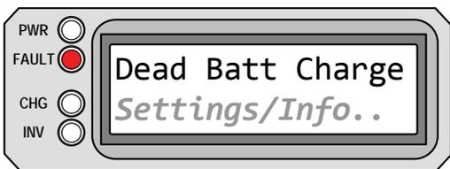
**Dead Batt Charge** appears on the LCD. The FAULT (red) LED is on. The PWR (green), CHG (green), and INV (green) LEDs are off.
