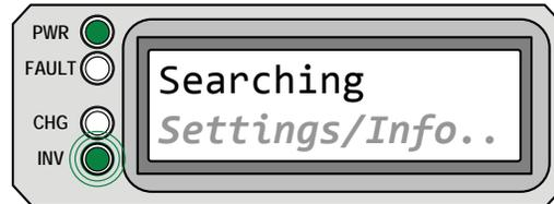
**Searching** appears on the LCD. The PWR (green) LED is on solid, and the INV (green) LED flashes. The FAULT (red) and CHG (green) LEDs are off.
