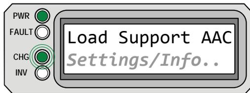
**Load Support AAC** appears on LCD. PWR (green) LED is on solid, and CHG (green) LED blinks. FAULT (red) LED is off, and INV (green) LED could be on or off.
