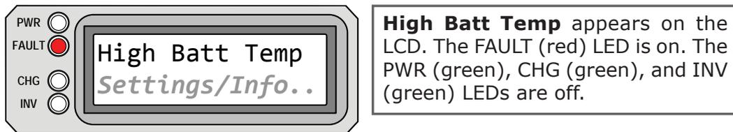
**Figure 5-23, High Battery Temperature Fault**
