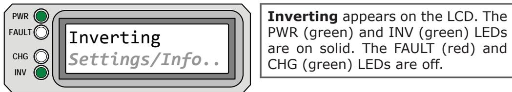
Figure 5-4, Inverting Mode
