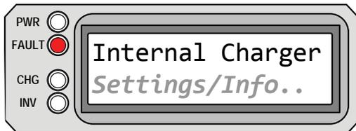
**Internal Charger** appears on the LCD. The FAULT (red) LED is on. The PWR (green), CHG (green), and INV (green) LEDs are off.
