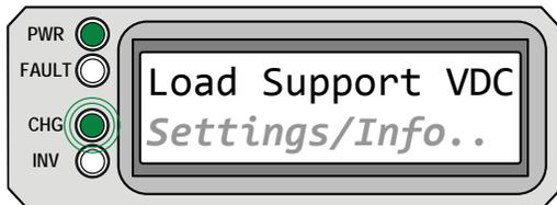
**Load Support VDC** appears on LCD. PWR (green) LED is on solid, and CHG (green) LED blinks. FAULT (red) LED is off, and INV (green) LED could be on or off.
