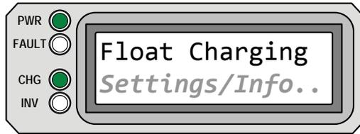
**Float Charging** appears on LCD. PWR (green) LED is on solid, and CHG (green) LED is on solid, but may blink. FAULT (red) LED is off, and INV (green) LED could be on or off.
