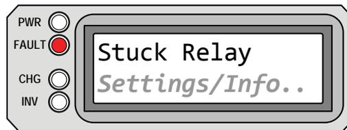
**Stuck Relay** appears on the LCD. The FAULT (red) LED is on. The PWR (green), CHG (green), and INV (green) LEDs are off.
