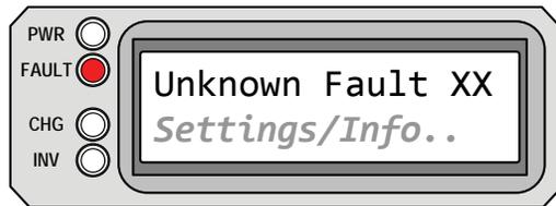
**Unknown Fault XX** appears on the LCD. The FAULT (red) LED is on. The PWR (green), CHG (green), and INV (green) LEDs are off.
