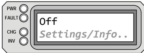
**Off** appears on the LCD. All LEDs are off.
