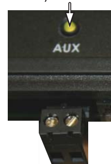
Aux Relay LED Indicator
