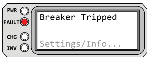
Figure 5-31, Breaker Tripped Fault
