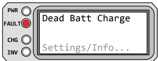
Figure 5-32, Dead Battery Charge Fault
