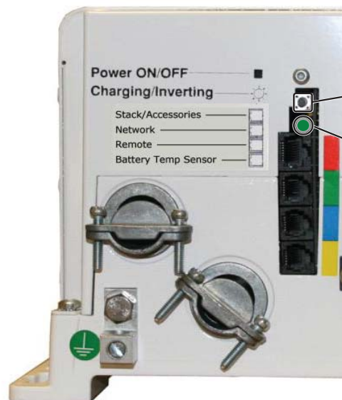
Figure 6-1, Performing an Inverter Reset
