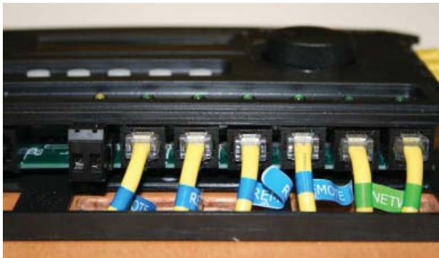
Figure 2-7, Concealed Mounted Remote/Network Cables
