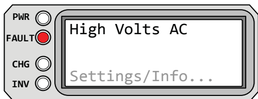
Figure 5-37, High Volts AC Fault
