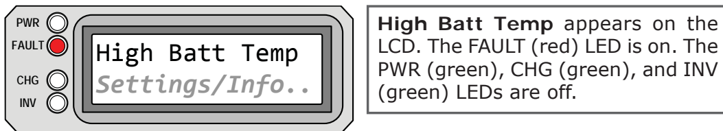
Figure 5-23, High Battery Temperature Fault
