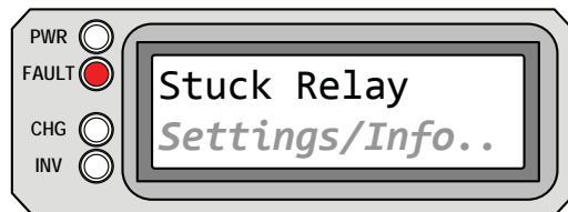
Figure 5-29, Stuck Relay Fault
