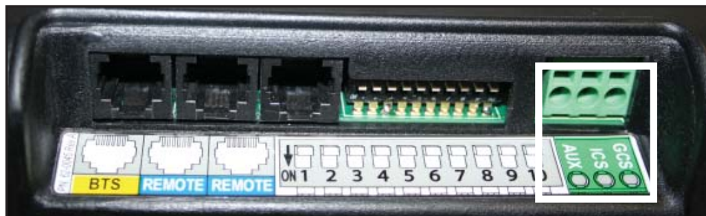
Figure 2-5, MMSA1012's 3-Port Terminal Block
