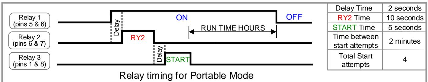
This diagram is provided to assist in the installation of the Auto Generator Start controller. Since the use of this diagram and the conditions or methods of installation, operation and use are beyond the control of Sensata Technologies (Magnum Energy Products), we do not assume responsibility and expressly disclaim liability for loss, damage or expense arising out of the installation, operation and use of this unit.
